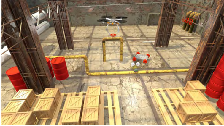
Figure 2: Heterogeneous symbiotic robotic system deployed on a mission to close a valve in a disaster stricken industrial environment
