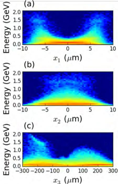
FIG. 4: Classical  $S$ -matrix projections for xLIPA electrons in the 10 PW case. The vertical axes are the final particle energies and the horizontal axes are the initial positions  $x_i$ , with laser polarization in the 1-direction and central wavevector in the 3-direction. High energies are encouraged by increasing the ion density near the two positions  $(x_1, x_2, x_3) \approx (\pm 7, 0, -200) \mu\text{m}$ .
