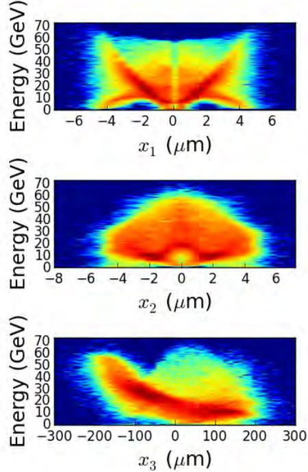
FIG. 6: Classical  $S$ -matrix projections for xLIPA electrons in the 25 EW case, neglecting radiation reaction. The vertical axes are the final particle energies and the horizontal axes are the initial positions  $x_i$ , with laser polarization in the 1-direction and central wavevector in the 3-direction. The vertical feature at  $x_1 = 0$  in (a) is an artifact of the initial particle loading.
