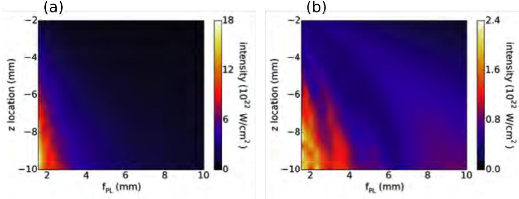
FIG. 11: Peak intensity as a function of plasma lens location, vertical axis, and plasma lens linear focal length, horizontal axis, for linear,  $\gamma \rightarrow 1$ , and nonlinear lenses. Even with the nonlinear aberrations, the peak intensity achieved by the plasma lens,  $\approx 2 \times 10^{22}$  W/cm<sup>2</sup>, surpasses that of the unassisted mirror,  $\approx 4 \times 10^{21}$  W/cm<sup>2</sup>.
