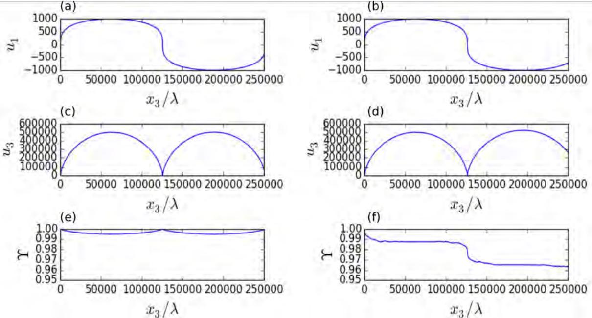
FIG. 7: Electron orbits in a plane wave without the reaction force (a,c,e) and with the exact Landau and Lifshitz reaction force (b,d,f). Here  $\Upsilon = u_0 - u_3$ , which is expected to be invariant in the absence of radiation reaction.
