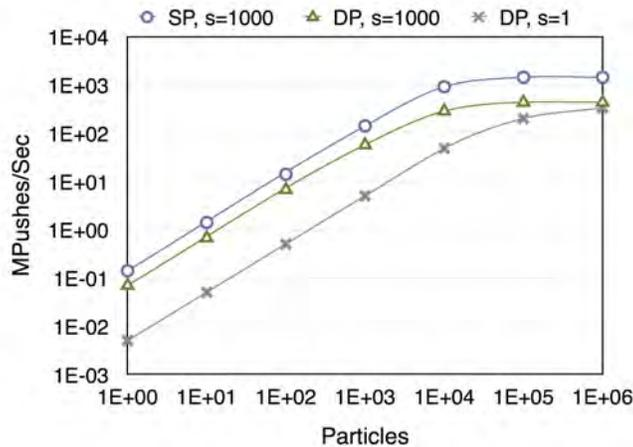
FIG. 10: Performance of covariant pusher, in terms of millions of particles advanced per second, including field evaluations. In the legend, SP means single precision, DP means double precision, and  $s$  is the number of cycles advanced for each OpenCL kernel invocation.
