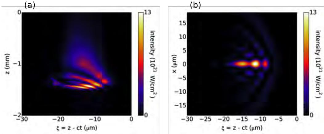
FIG. 12: (a) On-axis intensity as a function of distance in the speed of light frame, horizontal axis, and propagation distance, vertical axis. (b) The transverse intensity profile of the pulse at a propagation distance near where the pulse achieves its maximum intensity.
