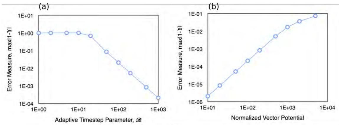
FIG. 9: Accuracy of covariant pusher, as measured by the maximum value of  $|1 - \Upsilon|$ , during one period of the motion of the electron in a plane wave. The accuracy is displayed as (a) a function of  $\mathcal{R}$ , given  $a_0 = 100$ , and (b) as a function of  $a_0$ , given  $\mathcal{R} = 1000$ . In all cases  $\Omega = 267$ .
