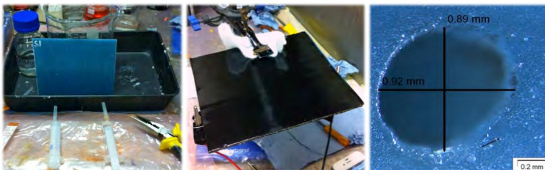
Fig 2.2. Softening PLA via resistive heating facilitates NiCr wire removal. Flush with solvent (CH<sub>3</sub>Cl) creating hollow vascules
