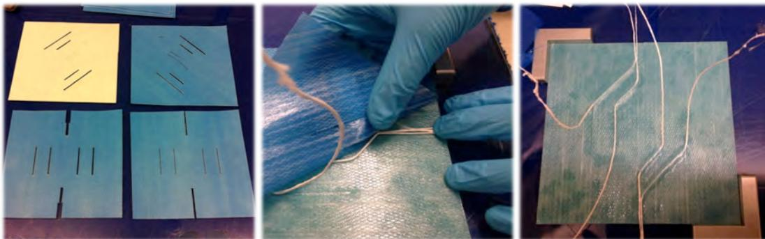
Fig 2.1. Hand layup of PLA coated NiCr wire into fibre direction cut-outs (SE70 Glass/epoxy prepeg)
