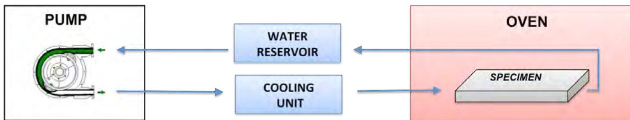
Fig. 2.6. Simplified schematic of the thermal ageing/active cooling system.
