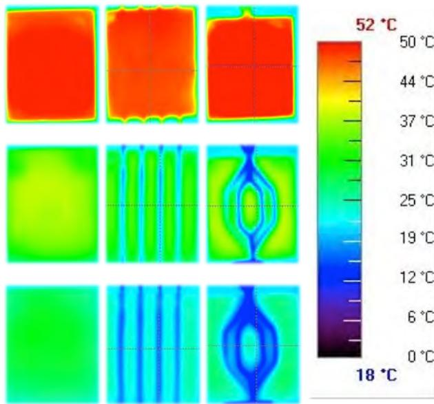
Fig. 2.3. Initial tests pumping water at 0°C through Ø0.9 mm vasculi at  $\approx$ 30ml/min show different performance of network designs (left) baseline, (centre) straight and (right) shape, after (a) 0 minutes (top), (b) 2 minutes (middle), (c) 5 minutes (lower).
