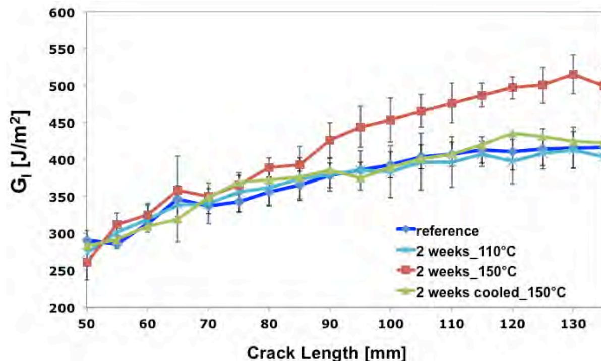
Fig. 2.11. Strain energy release rate ( $G_{IC}$ ) after 2 weeks of thermal ageing at 110°C, 150°C and while actively cooled at 150°C. Apparent toughness increase attributed to fibre bridging, clearly visible for specimens aged at 150°C.
