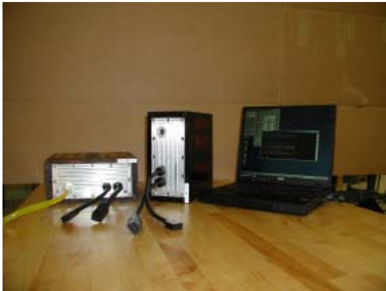
Figure 1: Batteries with charging computer. The cell stacks are encapsulated, while the intelligent controller sits in an oil filled cavity at one end. This cavity has an aluminum lid with external wires through liquid tight fittings.
