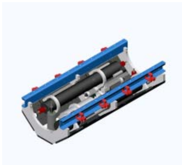
[Exploded view of payload mid-section of AUV, showing sensor layout]
