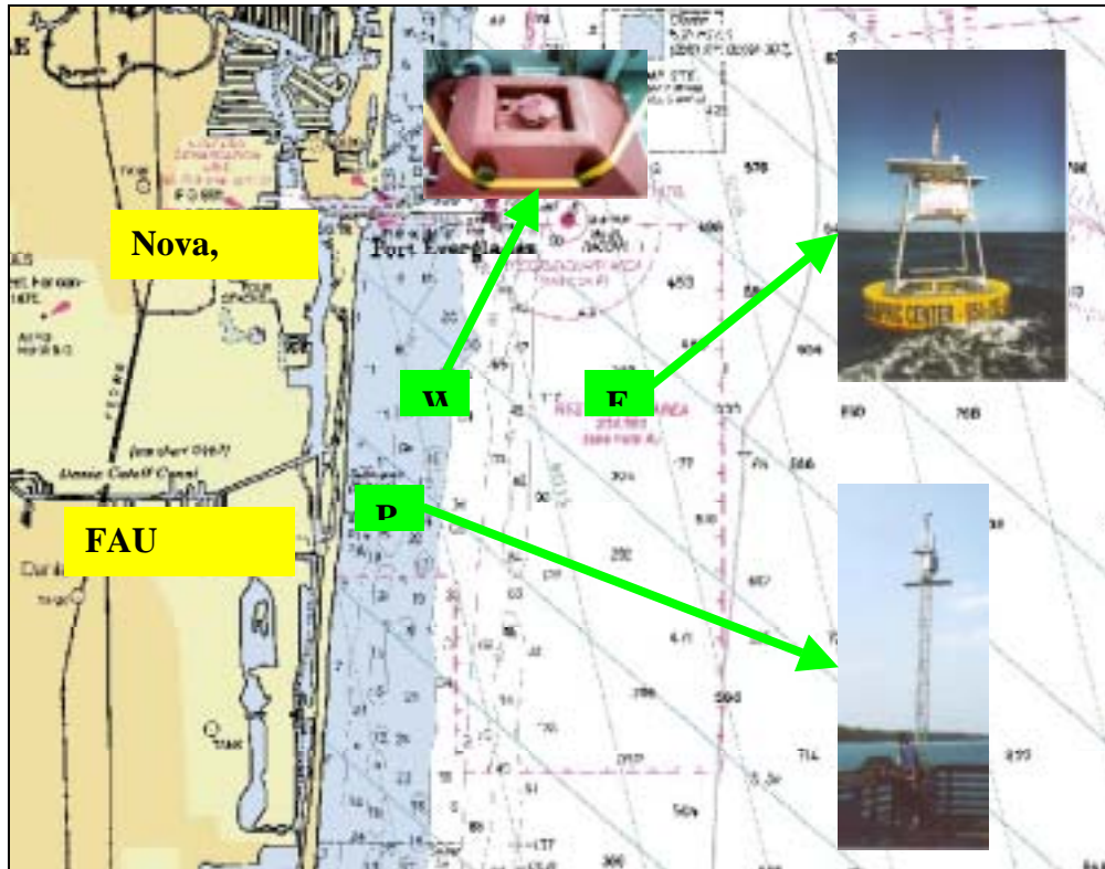
Figure 1. The NSU/USF Environmental Array in the SFOMC experimental range during Year 4. Here: W is the west (bottom) mooring, E the East Mooring, and P the Dania Pier meteorological station.
