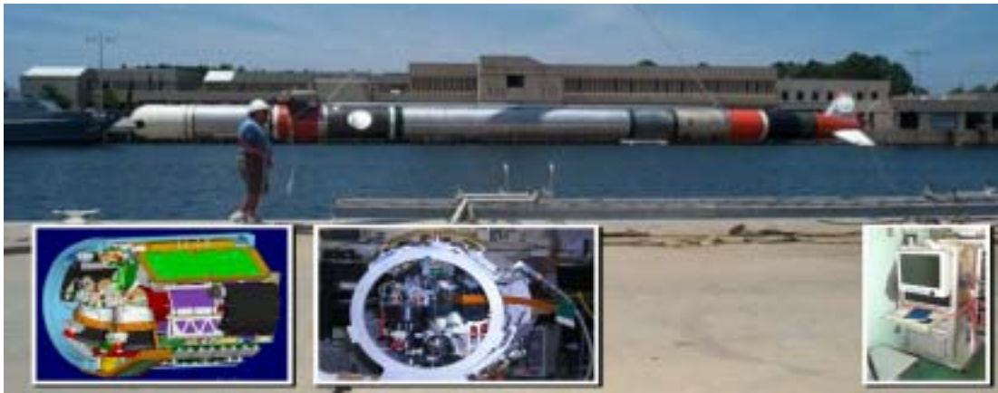
Figure 1: STIL, Processing System, and EOID Multi-sensor Tow Body [Tow body shown dockside with STIL sensor integrated in small section ahead of the tow body wing. STIL CAD drawing. STIL Sensor in Laboratory. Topside processing system as deployed onboard ship]
