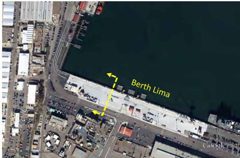
Figure 4-277. Google Earth aerial view showing the configuration of Berth Lima and Quay Road, NBC. The dashed yellow line indicates the approximate location of the storm drain section shown in Figure 4-277 (image: Google).
