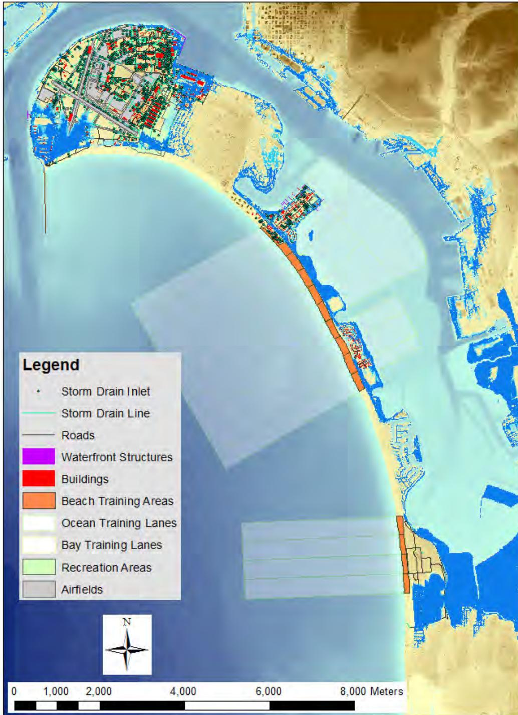
Figure 4-121. Inundation and flooding for the 2.0-m SLR bay-exposure scenario at NBC. The blue shaded zones represent week (dark blue), year (medium blue), and century (light blue) return periods.
