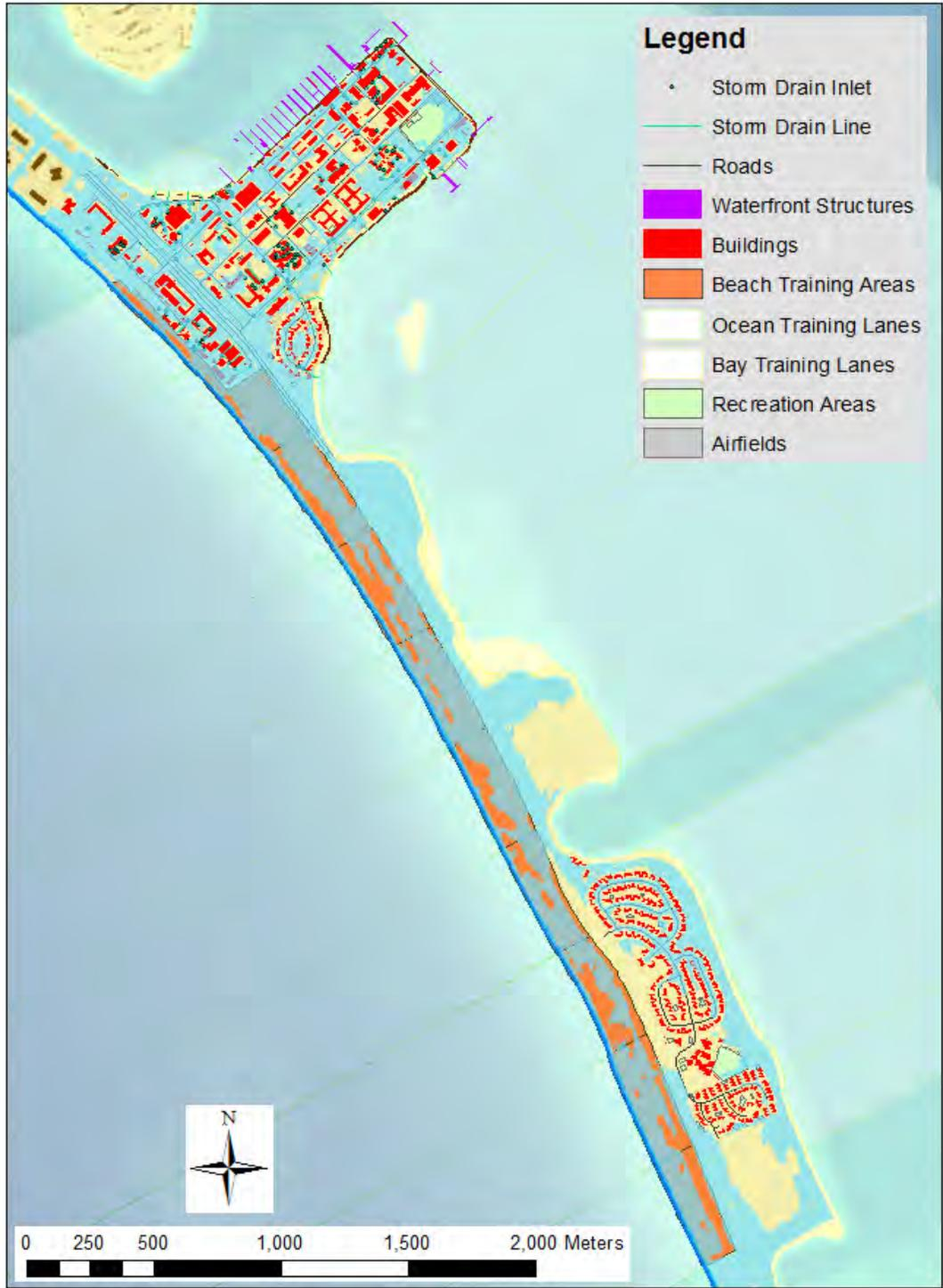
Figure 4-90. Detailed view of inundation and flooding for the baseline (SLR = 0 m) scenario at NAB/STTC North. The blue shaded zones represent week (dark blue), year (medium blue), and century (light blue) return periods.
