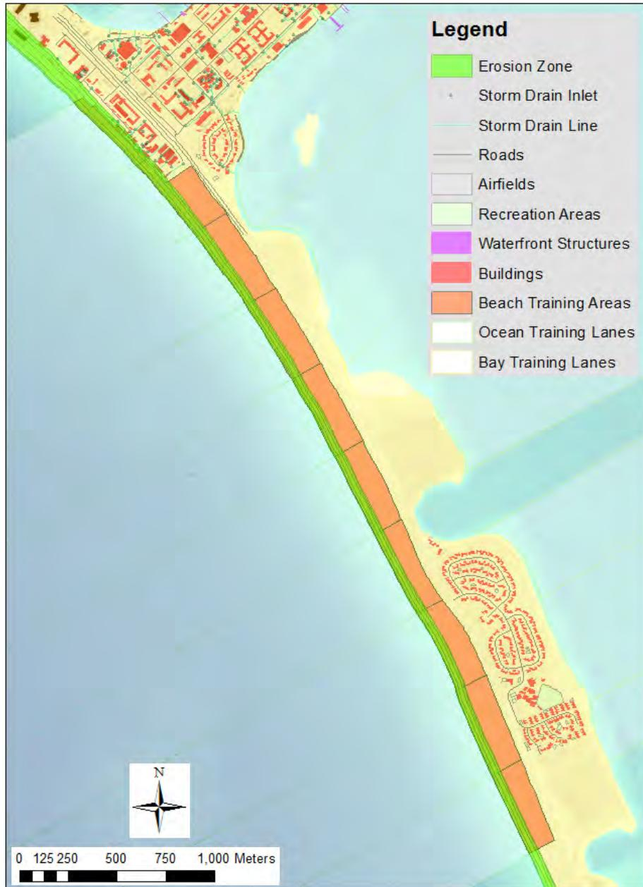
Figure 4-61. Detailed view of the erosion footprint for the baseline (SLR = 0 m) scenario at NAB/SSTC North. The overall green shaded band spans the 100r year return period wave condition from the YGOR model, and the fine grey lines indicate the shorter return periods ranging from week to decade.
