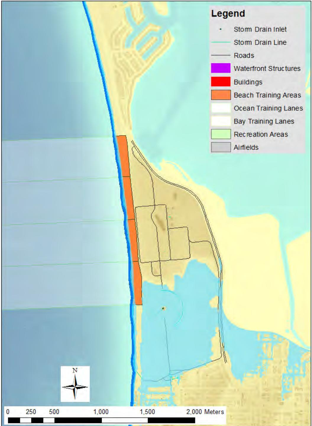
Figure 4-91. Detailed view of inundation and flooding for the baseline (SLR = 0 m) scenario at STTC South. The blue shaded zones represent week (dark blue), year (medium blue), and century (light blue) return periods.
