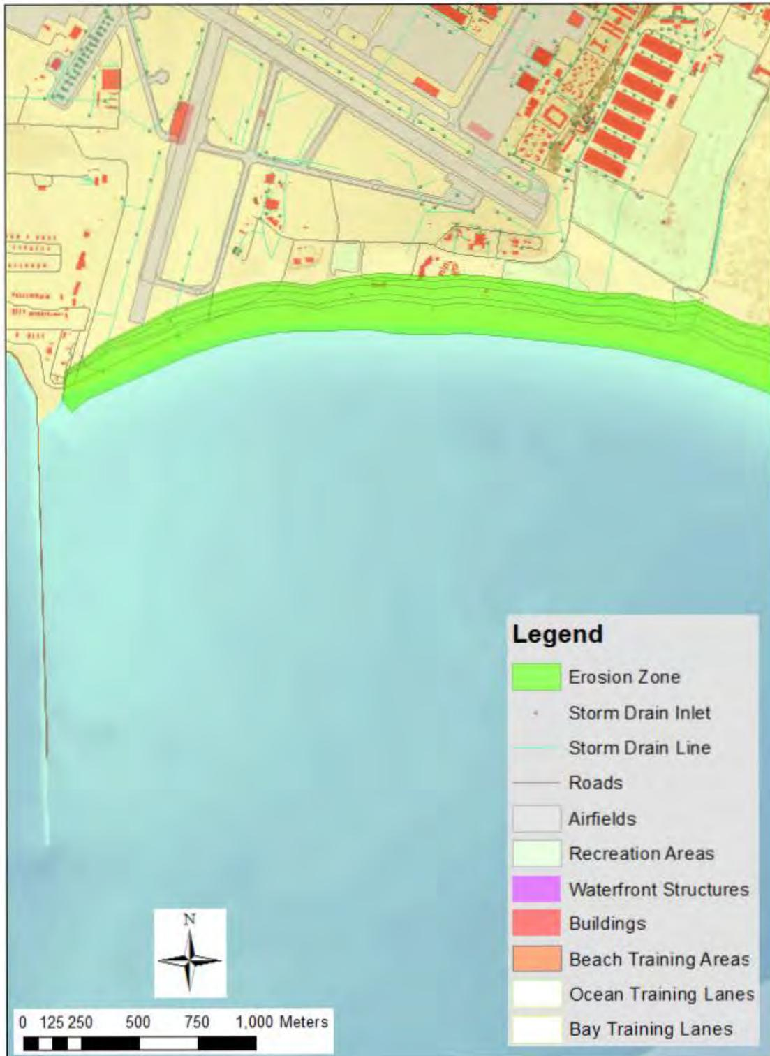
Figure 4-68. Detailed view of the erosion footprint for the SLR = 2.0-m scenario at North Island. The overall green shaded band spans the 100-year return period wave condition from the YGOR model, and the fine grey lines indicate the shorter return periods ranging from week to decade.
