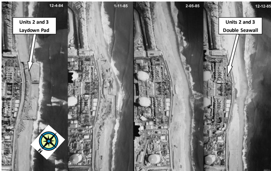
Figure 2-27. Composite of four aerial photographs of SONGS Units 2 and 3 taken near the end of construction between 4 December 1984, just before removal of the Units 2 and 3 laydown pad began (left), and 12 December 1985 (right) after beach had begun narrowing. The pad had been in place from 1974–1984 (courtesy of Southern California Edison Company; see Flick *et al.*, 2010; note the photo orientation with ocean on the right).
