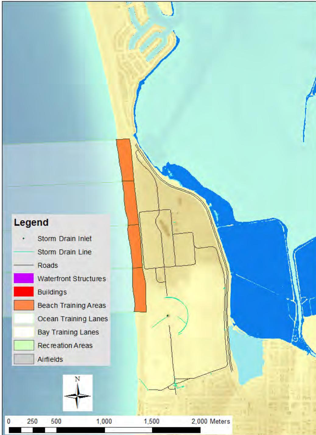
Figure 4-116. Detailed view of inundation and flooding for the baseline (SLR = 0 m) bay-exposure scenario at SSTC South. The blue shaded zones represent week (dark blue), year (medium blue), and century (light blue) return periods.
