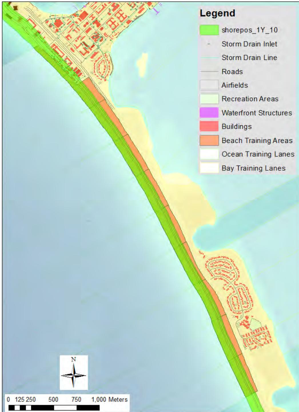
Figure 4-65. Detailed view of the erosion footprint for the SLR = 1.0-m scenario at NAB/SSTC North. The overall green shaded band spans the 100-year return period wave condition from the YGOR model, and the fine grey lines indicate the shorter return periods ranging from week to decade.
