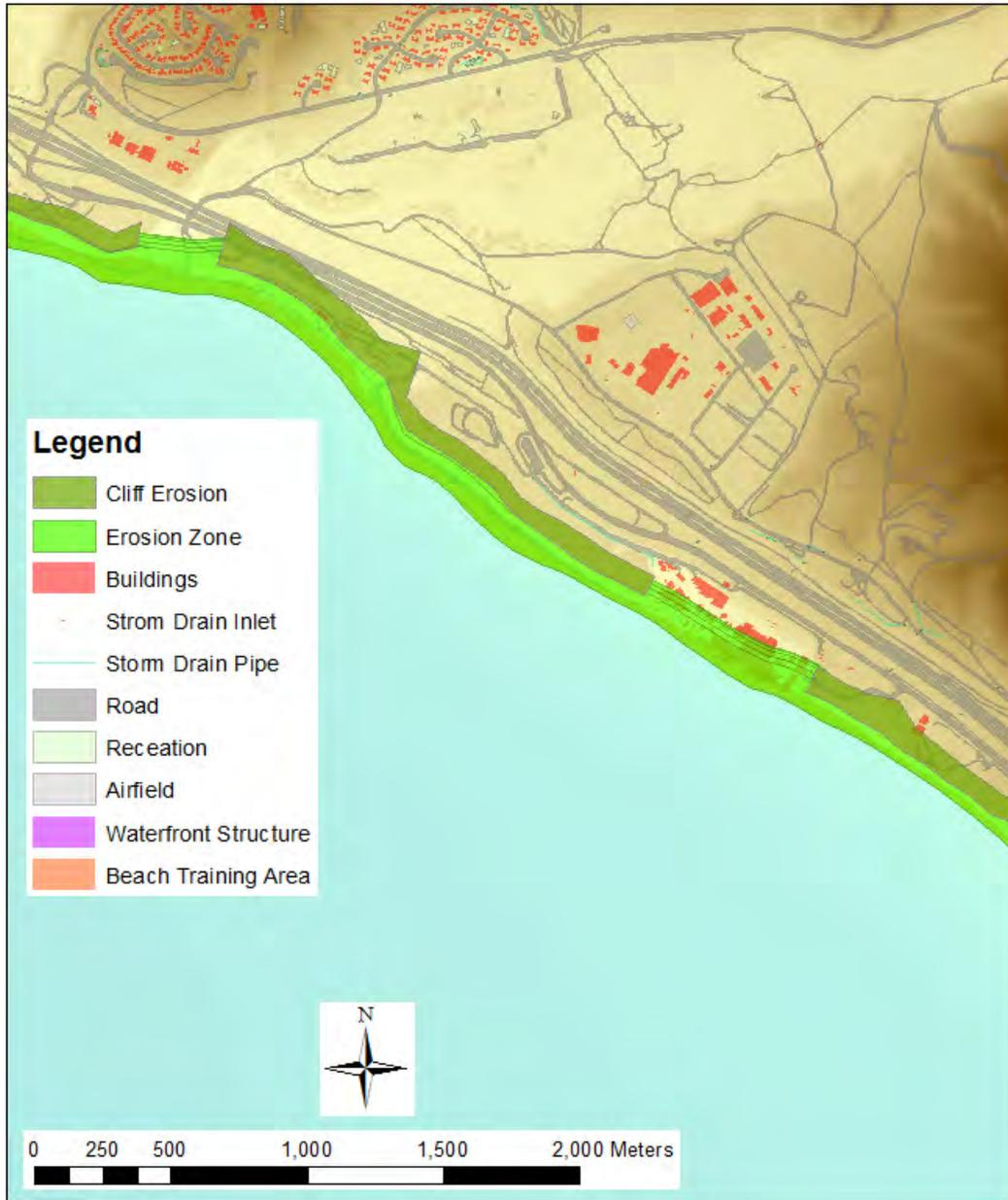
Figure 4-86. Detailed view of the erosion footprint for the SLR = 2.0-m scenario at San Onofre. The overall light green shaded band spans the 100-year return period wave condition from the YGOR model, and the fine grey lines indicate the shorter return periods ranging from week to decade. The dark green shaded band indicates the extent of cliff erosion.
