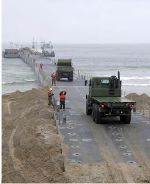
Figure 4-224. Elevated Causeway System training activity. The causeway is anchored to shore, and extends beyond the surf zone (U.S. Navy photo by Mass Communication Specialist 2nd Class Bryan Niegel).
