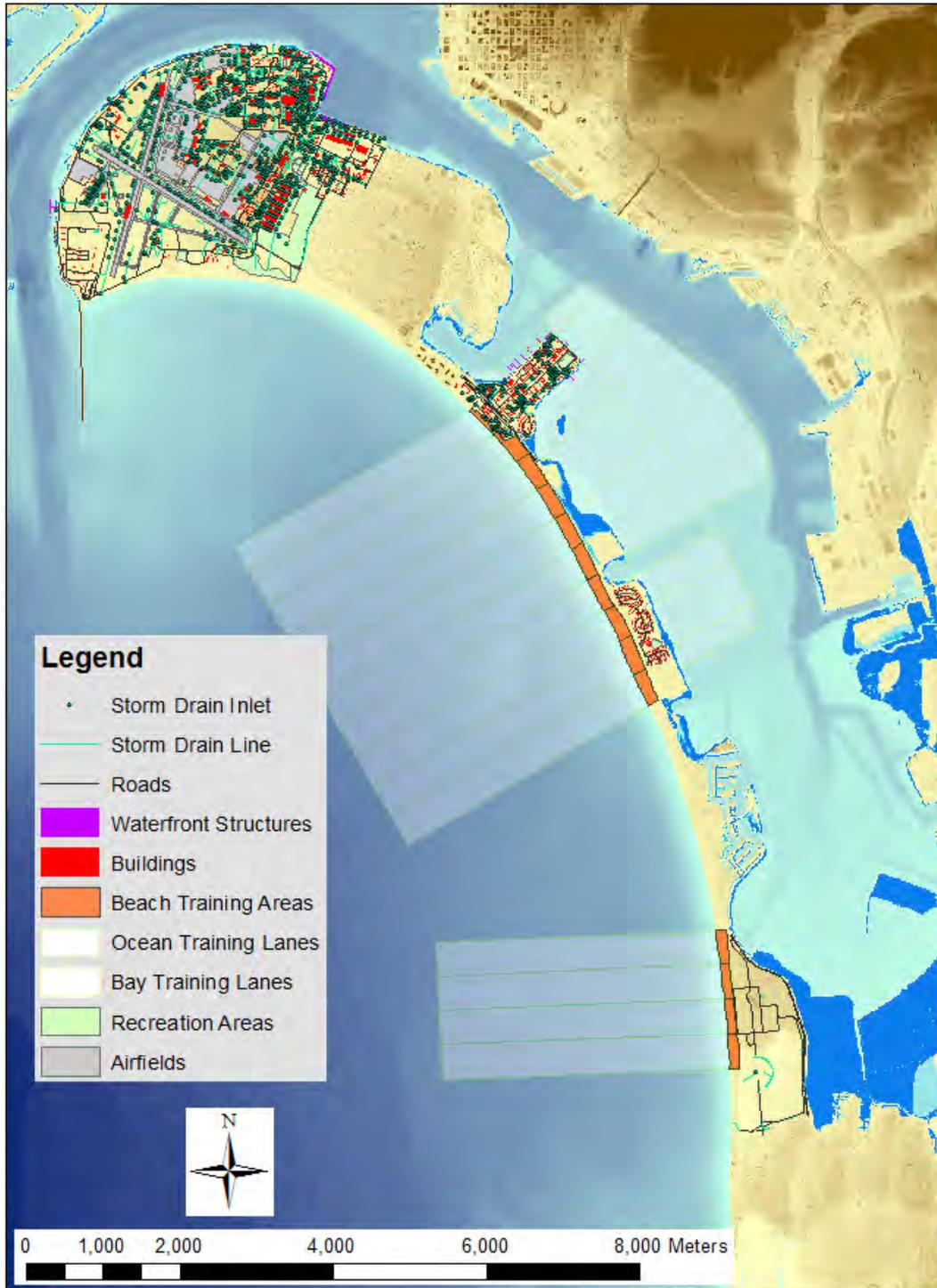
Figure 4-117. Inundation and flooding for the 1.0-m SLR bay-exposure scenario at NBC. The blue shaded zones represent week (dark blue), year (medium blue), and century (light blue) return periods.
