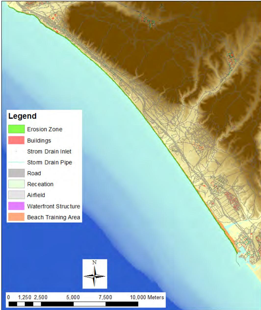
Figure 4-75. Erosion footprint for the baseline (SLR = 0 m) scenario at MCBCP. The overall light green shaded band spans the 100-year return period wave condition from the YGOR model, and the fine grey lines indicate the shorter return periods ranging from week to decade.
