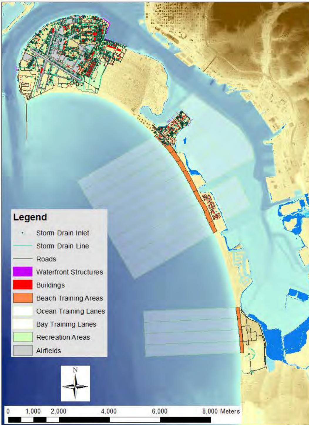
Figure 4-113. Inundation and flooding for the baseline (SLR = 0 m) bay-exposure scenario at NBC. The blue shaded zones represent week (dark blue), year (medium blue), and century (light blue) return periods.
