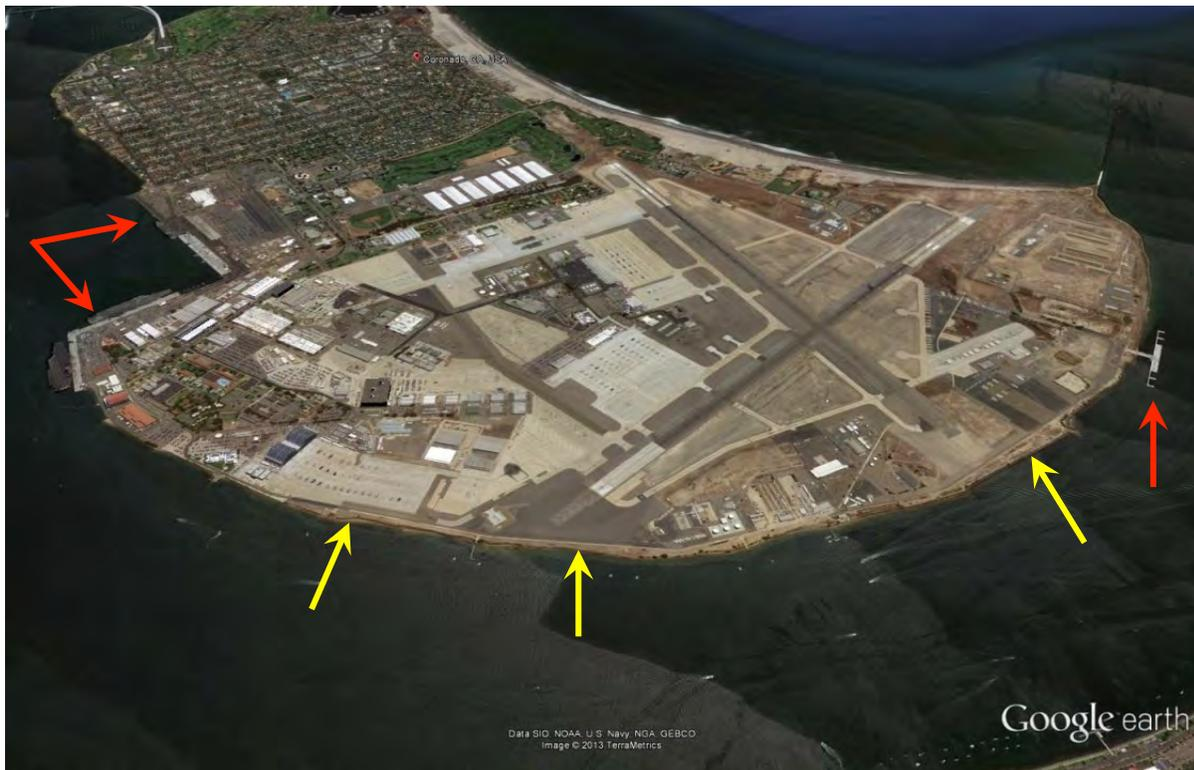
Figure 3-46. Waterfront structures at NBC including the Carrier Wharves (far left) and the Ammunition Pier (far right) (red arrows). Shore protection coastal structures can also be seen along the bay shoreline (yellow arrows) (image data: Google).
