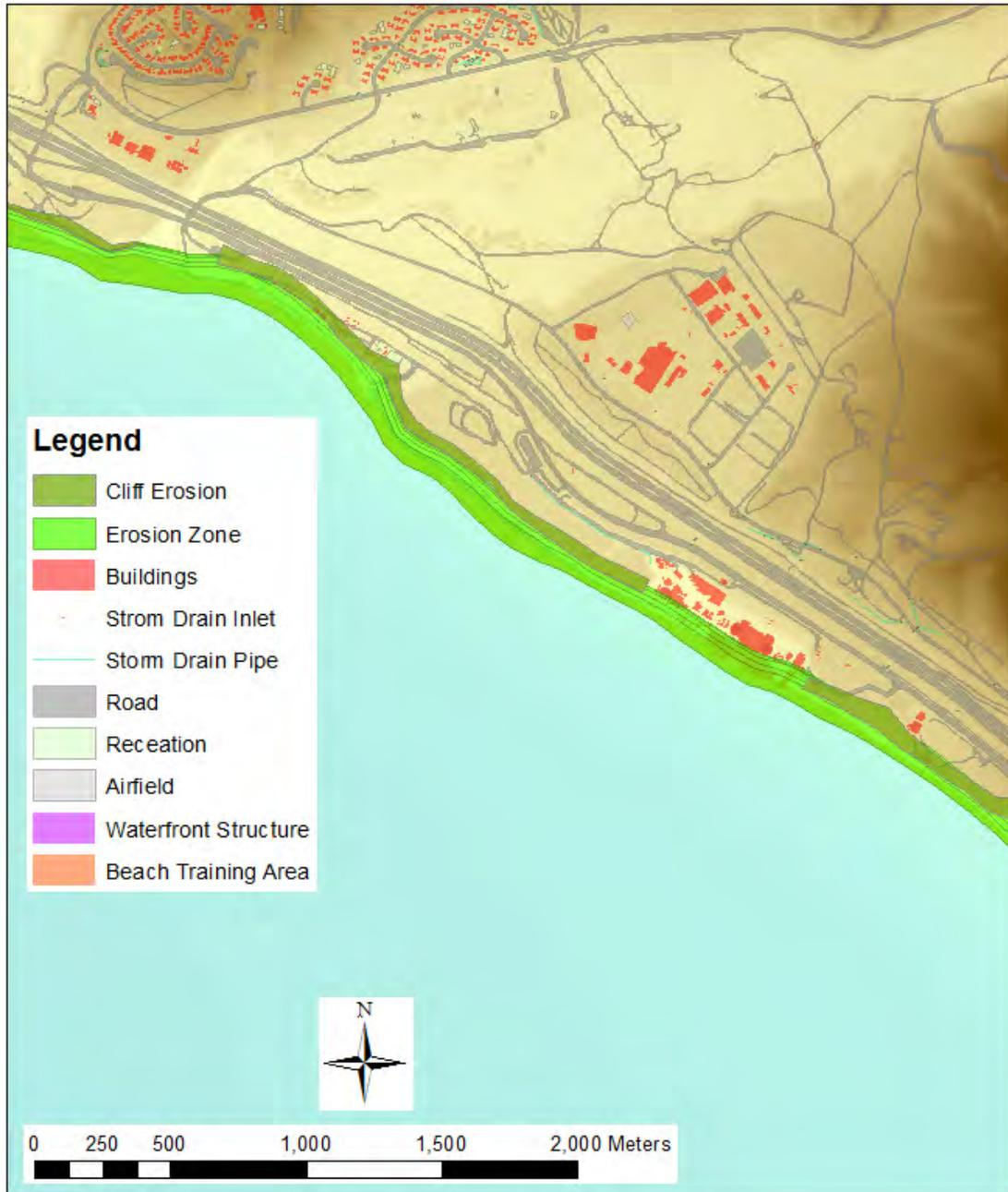
Figure 4-82. Detailed view of the erosion footprint for the SLR = 1.0-m scenario at San Onofre. The overall light green shaded band spans the 100-year return period wave condition from the YGOR model, and the fine grey lines indicate the shorter return periods ranging from week to decade. The dark green shaded band indicates the extent of cliff erosion.
