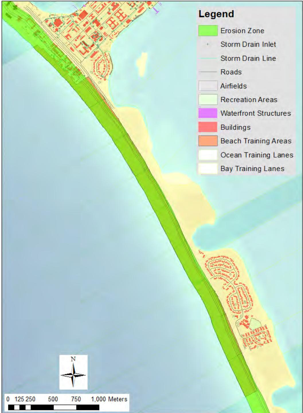
Figure 4-69. Detailed view of the erosion footprint for the SLR = 2.0-m scenario at NAB/SSTC North. The overall green shaded band spans the 100-year return period wave condition from the YGOR model, and the fine grey lines indicate the shorter return periods ranging from week to decade.
