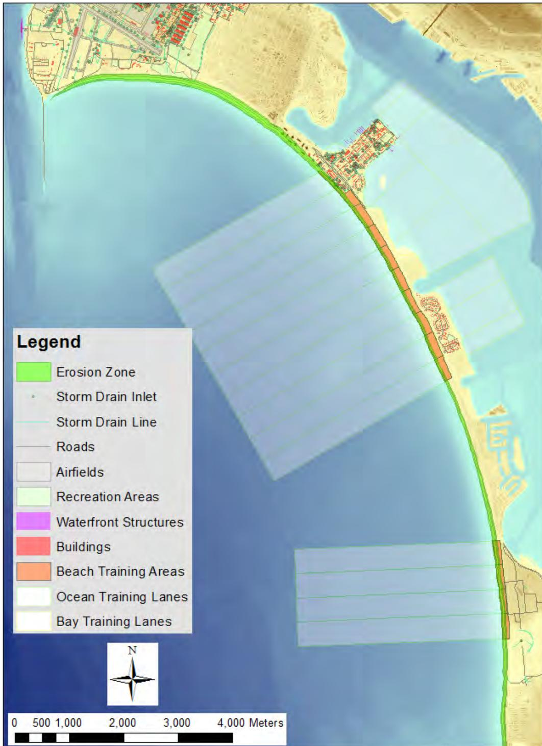
Figure 4-59. Erosion footprint for the baseline (SLR = 0 m) scenario at NBC. The overall green shaded band spans the 100-year return period wave condition from the YGOR model, and the fine grey lines indicate the shorter return periods ranging from week to decade.
