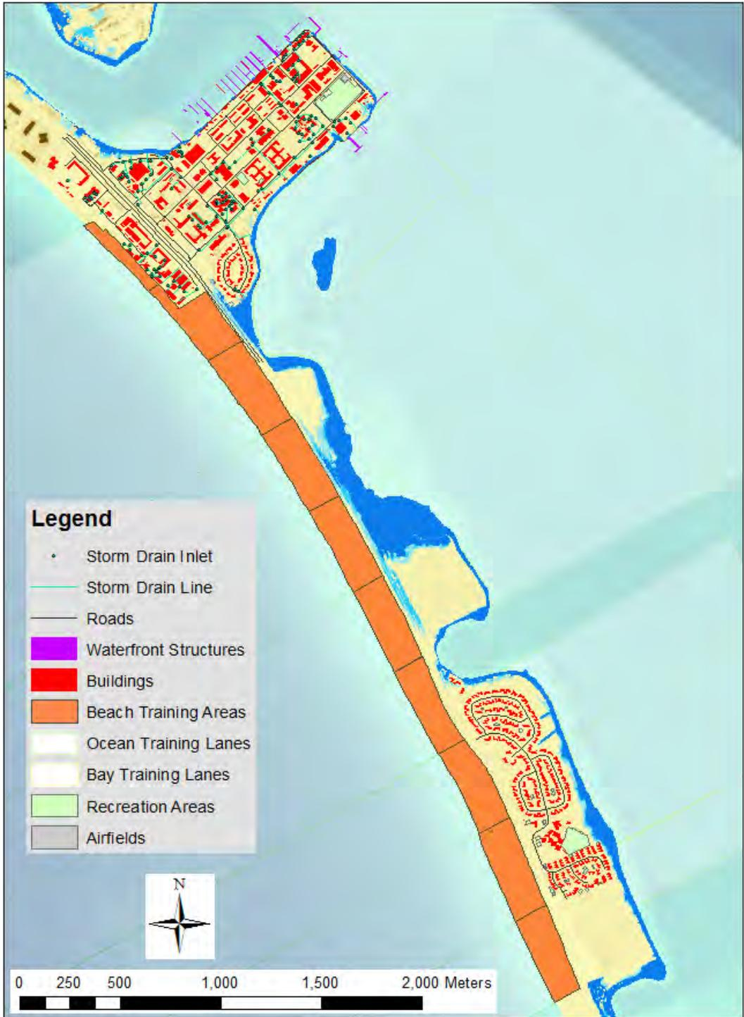
Figure 4-119. Detailed view of inundation and flooding for the 1.0-m SLR bay-exposure scenario at NAB/SSTC North. The blue shaded zones represent week (dark blue), year (medium blue), and century (light blue) return periods.
