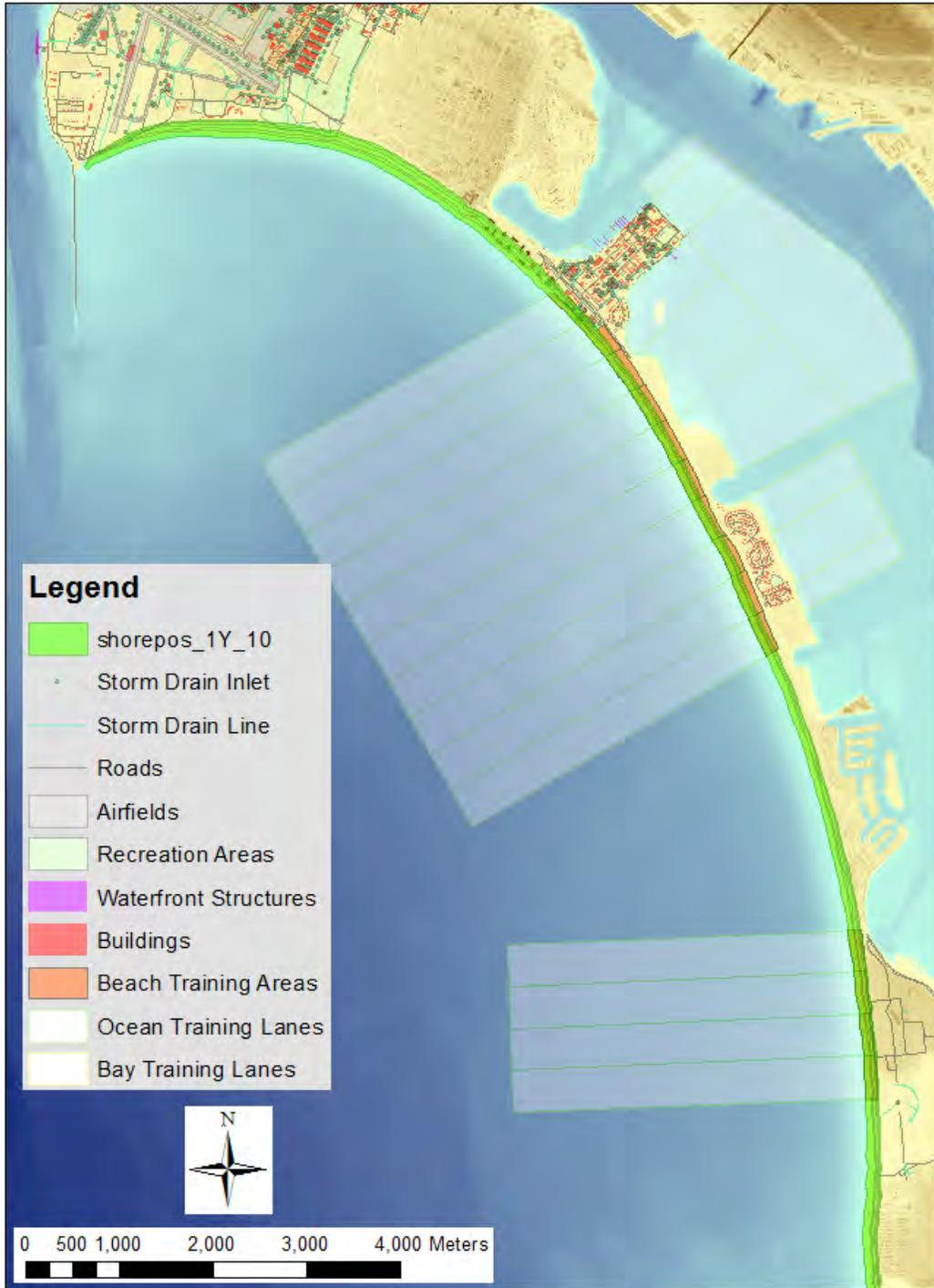
Figure 4-63. Erosion footprint for the SLR = 1.0-m scenario at NBC. The overall green shaded band spans the 100-year return period wave condition from the YGOR model, and the fine grey lines indicate the shorter return periods ranging from week to decade.
