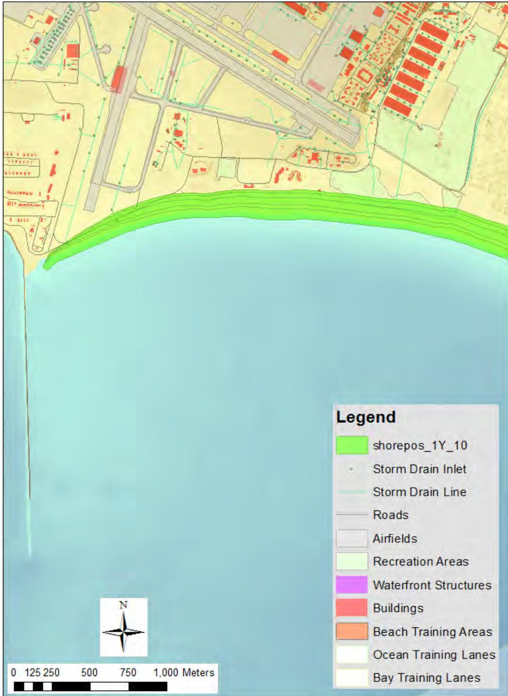
Figure 4-64. Detailed view of the erosion footprint for the SLR = 1.0-m scenario at North Island. The overall green shaded band spans the 100-year return period wave condition from the YGOR model, and the fine grey lines indicate the shorter return periods ranging from week to decade.
