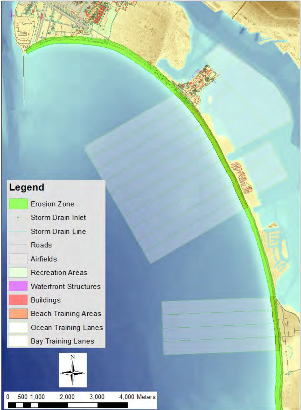
Figure 4-67. Erosion footprint for the SLR = 2.0-m scenario at NBC. The overall green shaded band spans the 100-year return period wave condition from the YGOR model, and the fine grey lines indicate the shorter return periods ranging from week to decade.
