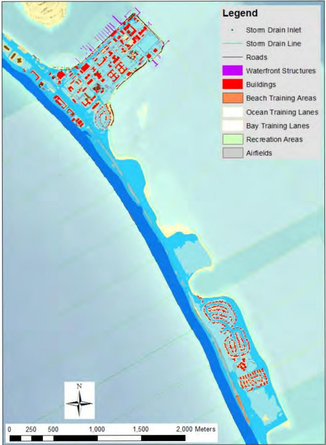
Figure 4-94. Detailed view of inundation and flooding for the SLR = 1.0 m scenario at NAB/STTC North. The blue shaded zones represent week (dark blue), year (medium blue), and century (light blue) return periods.
