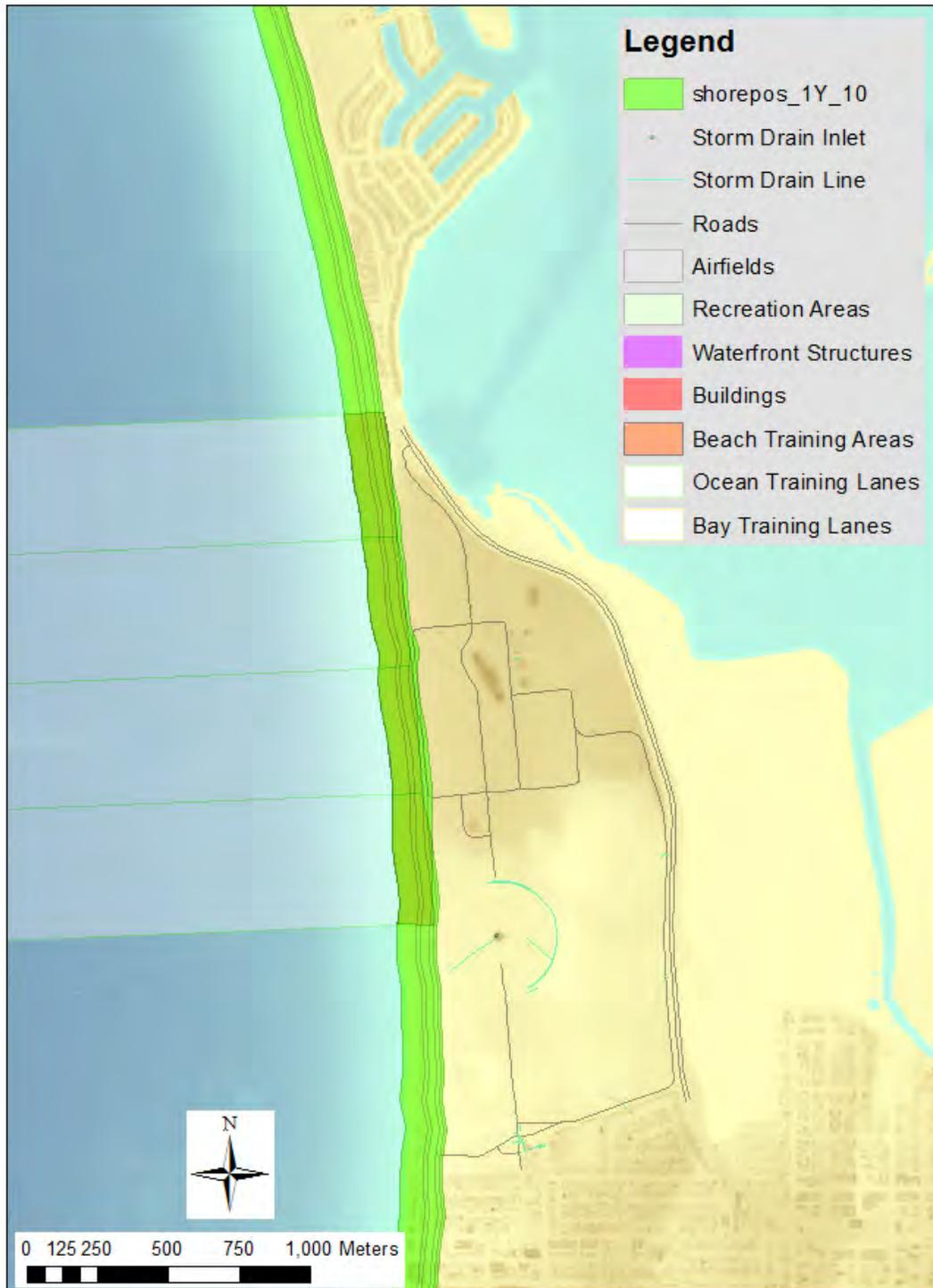
Figure 4-66. Detailed view of the erosion footprint for the SLR = 1.0-m scenario at SSTC South. The overall green shaded band spans the 100-year return period wave condition from the YGOR model, and the fine grey lines indicate the shorter return periods ranging from week to decade.
