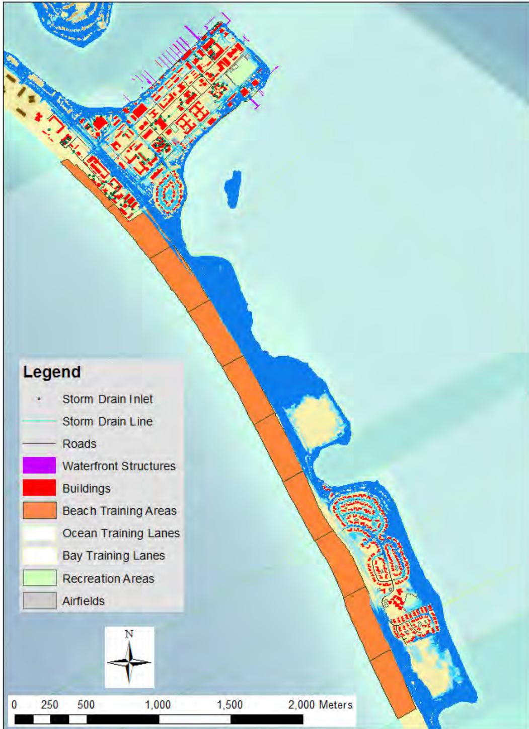
Figure 4-123. Detailed view of inundation and flooding for the 2.0-m SLR bay-exposure scenario at NAB/SSTC North. The blue shaded zones represent week (dark blue), year (medium blue), and century (light blue) return periods.
