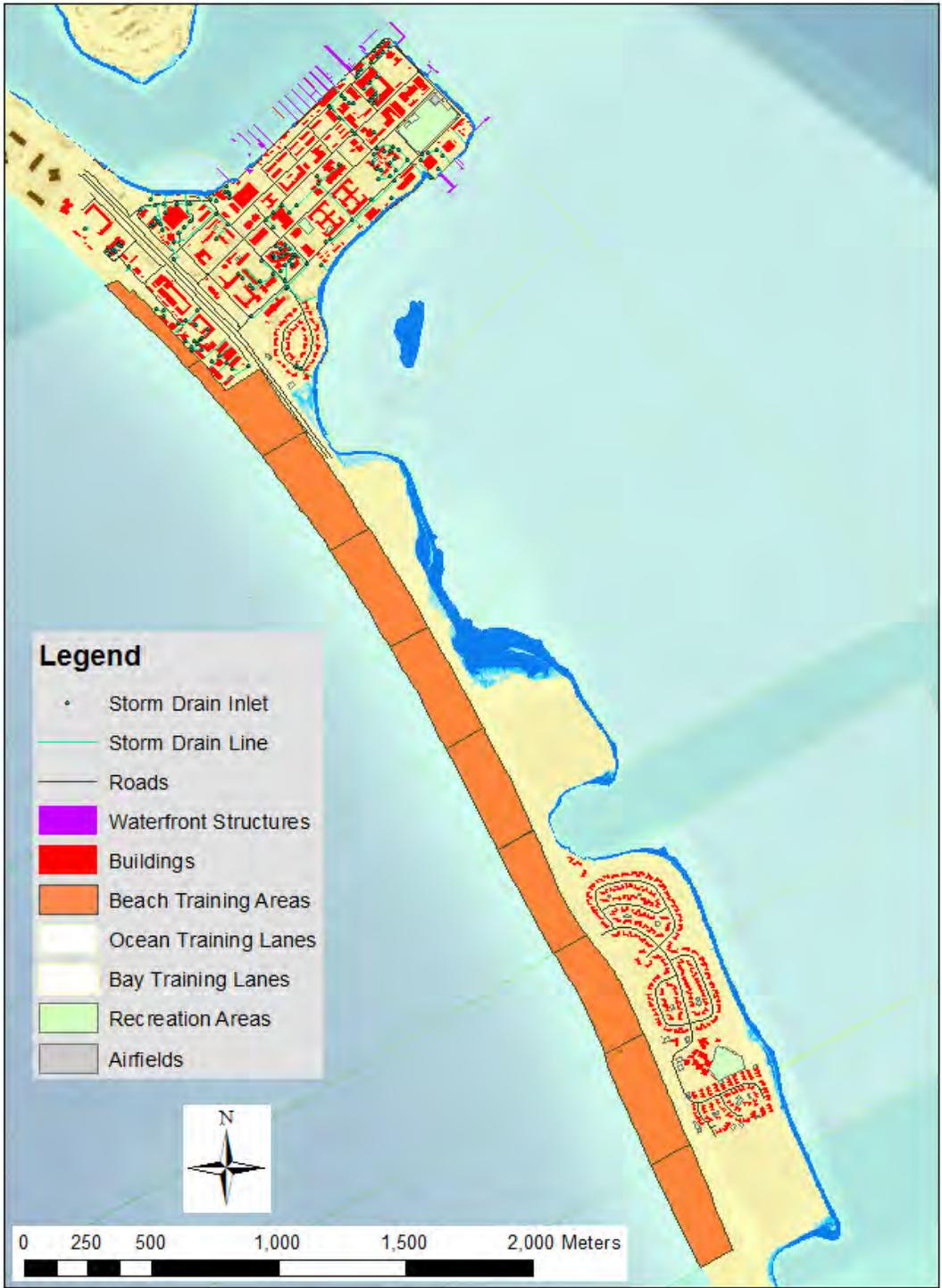
Figure 4-115. Detailed view of inundation and flooding for the baseline (SLR = 0 m) bay-exposure scenario at NAB/SSTC North. The blue shaded zones represent week (dark blue), year (medium blue) and century (light blue) return periods.
