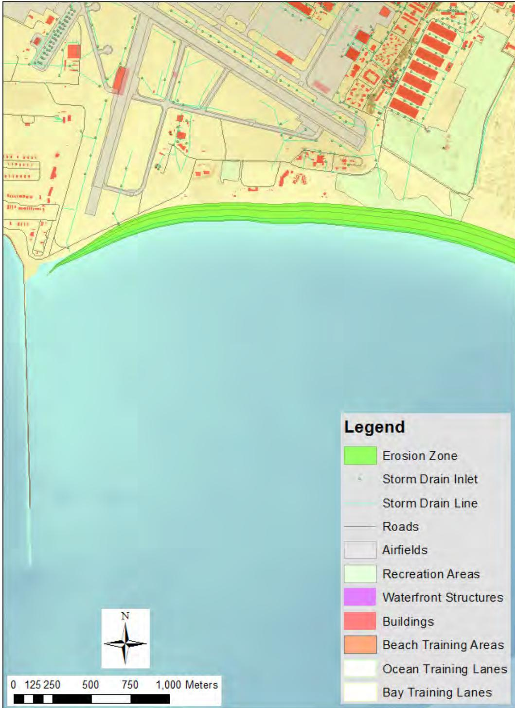
Figure 4-60. Detailed view of the erosion footprint for the baseline (SLR = 0 m) scenario at North Island. The overall green shaded band spans the 100-year return period wave condition from the YGOR model, and the fine grey lines indicate the shorter return periods ranging from week to decade.
