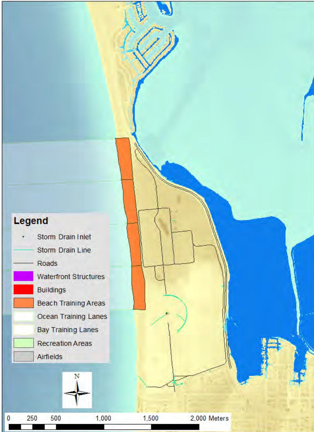
Figure 4-120. Detailed view of inundation and flooding for the 1.0-m SLR bay-exposure scenario at SSTC South. The blue shaded zones represent week (dark blue), year (medium blue), and century (light blue) return periods.
