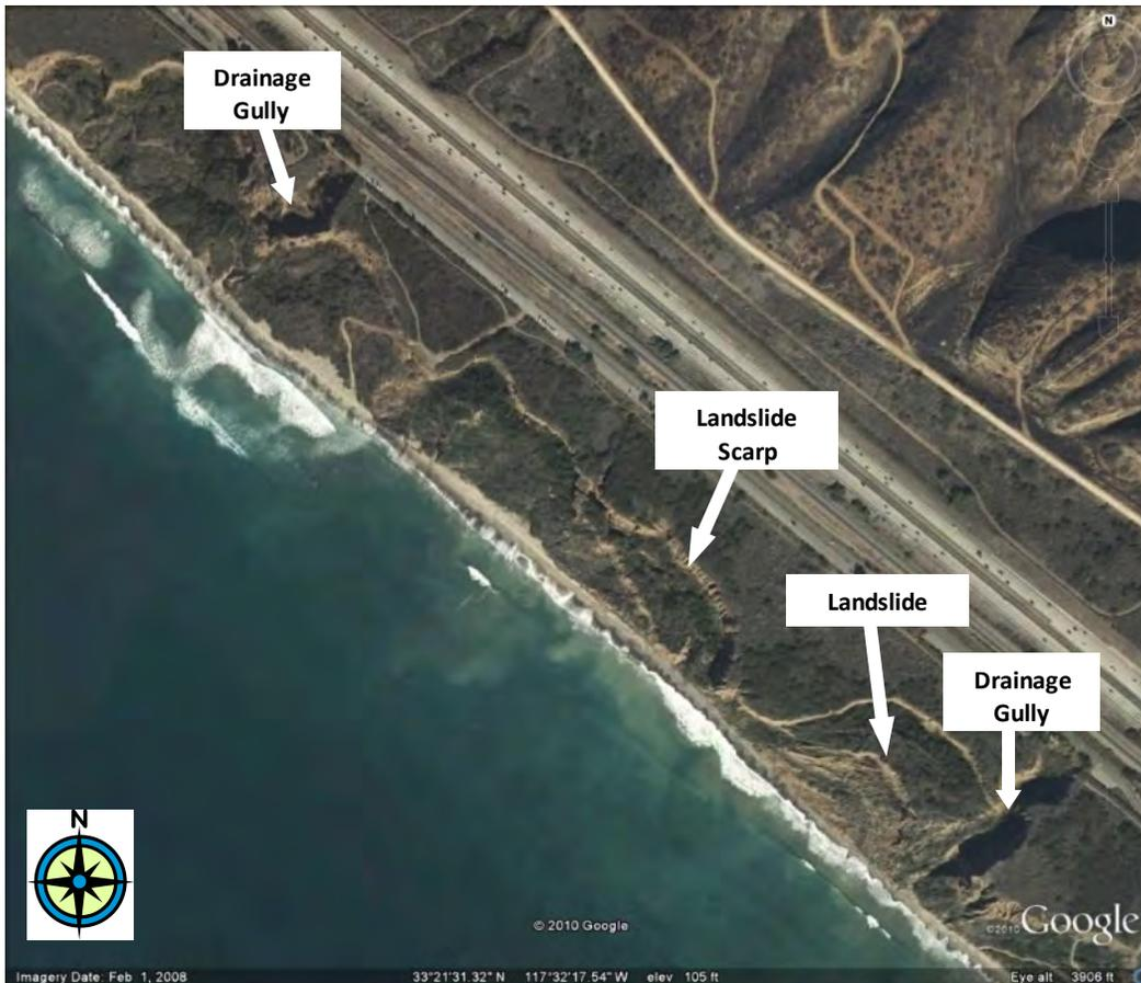
Figure 2-29. Google Earth image taken 1 February 2008 of 2 km of coast south of SONGS shows narrow, cliff-backed beach with landslides and several large gullies associated with drainage culverts and channels (see text).
