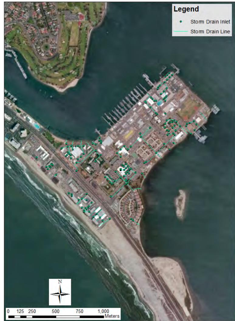
Figure 4-45. Detailed view of the storm water system at North Island (left) and NAB (right).
