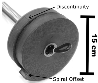
FIG. 1. Photograph of spiral wave front beacon prototype. The circular reference source is at the top and the spiral source is at the bottom. The discontinuity in the transducer material and the spiral offset are indicated.
