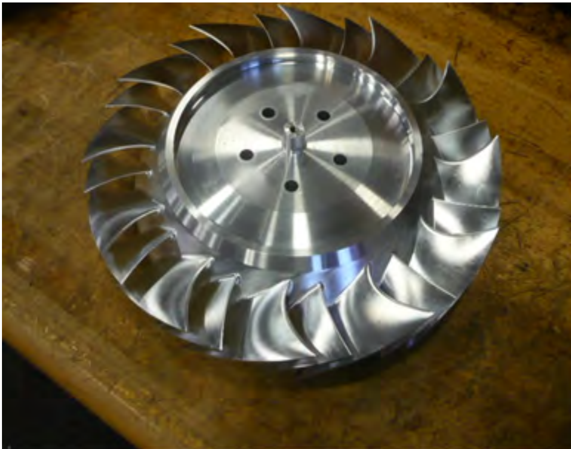
Fig. 24, Final machined TASR blisk
