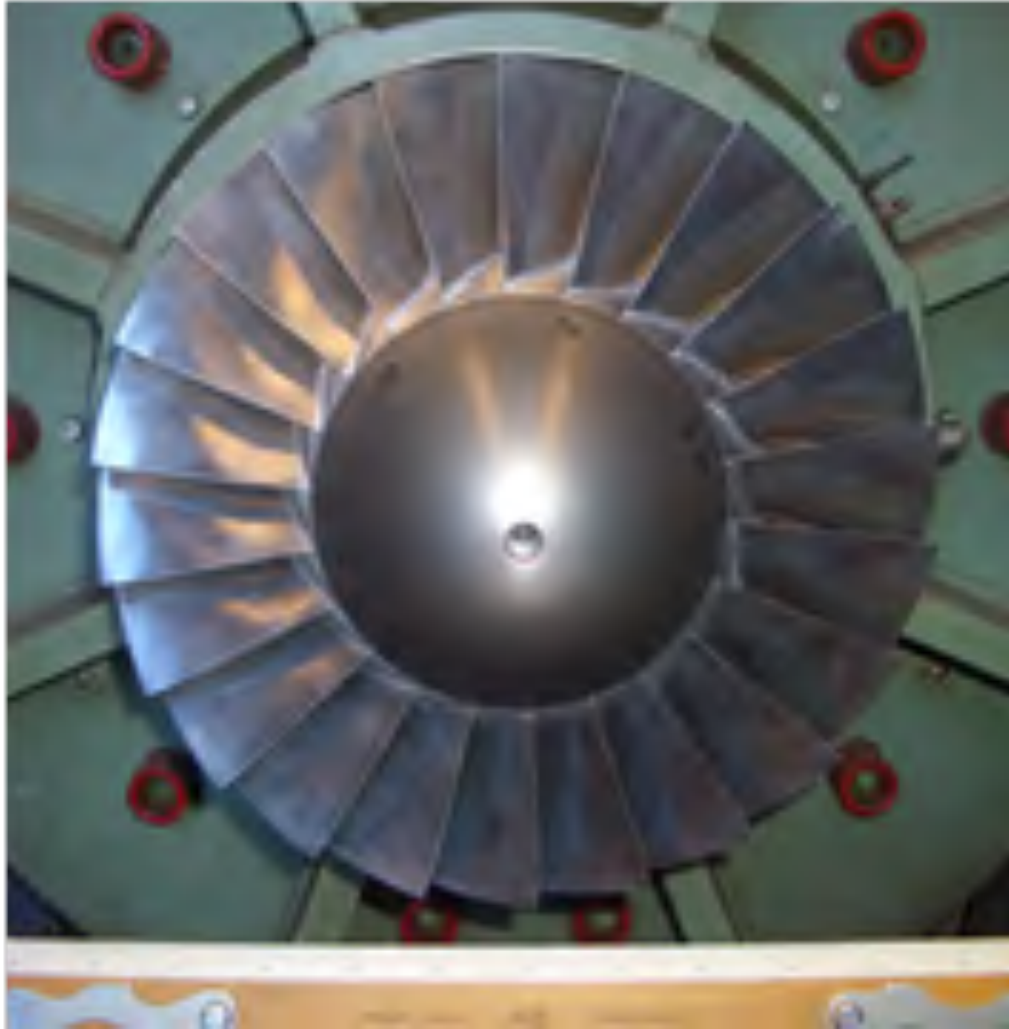
Fig. 4, Sanger's transonic axial compressor rotor [17].
