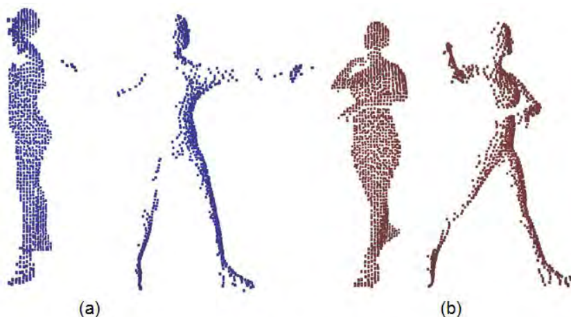
Figure 1. Simulated LIDAR Point Clouds
