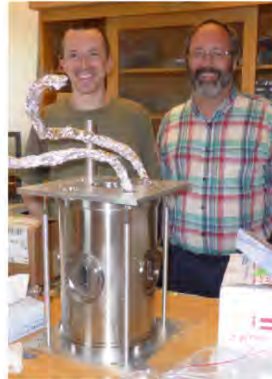
Figure 19: The leak tight Ti vacuum enclosure within which the low inductance Ioffe trap is located, with Eric Tardiff (the postdoc who championed this very difficult project) and the PI.
