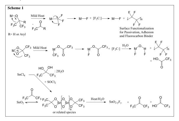
Although precursor compounds with  $M = Sn^{+4}$  were made, it was found that the more electron withdrawing nature of this metal relative to K<sup>+</sup> and Na<sup>+</sup> stabilized the starting material and decomposition required higher temperatures (> 150°C) to occur. We were encouraged, however, by the fact that at these high temperatures (400°C) transparent films were formed with low surface resistivity ( $\rho_s \approx 35 \Omega/sq$ ).
