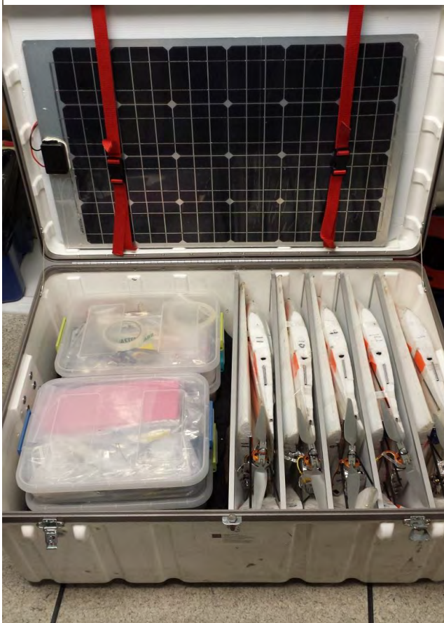
Figure 1: Assembled DataHawk 2 aircraft, shown on top of the DataHawk Flock Pod shipping case. Wing span is 52in., gross weight is 1.1Kg, flight speed ranges between 12 and 24 m/s, and duration in level flight is about 100 minutes.
