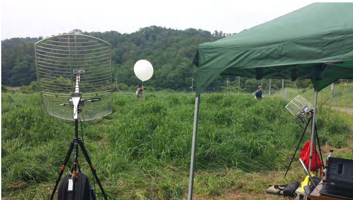
Figure 4: Preparing for a weather balloon drop deployment of the DataHawk 2 at Shigaraki. This enabled flights up to about 4km above ground level. For these higher flights, higher gain antennas are needed (left). Both 2.4 GHz and 900 MHz ISM bands have been used. 2.4 GHz was necessary in Japan due to frequency restrictions there.
