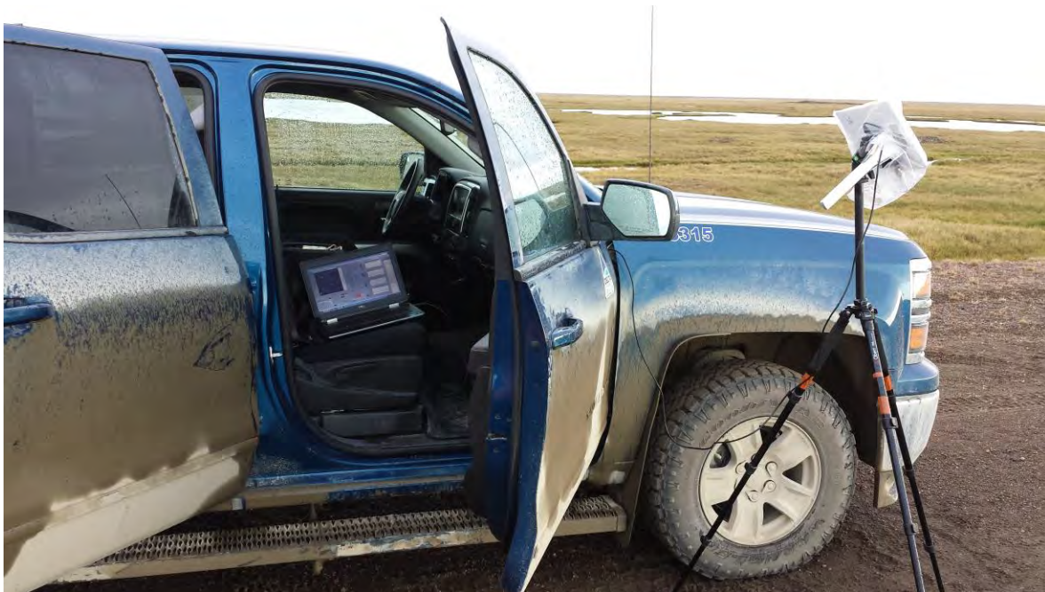
Figure 7: DataHawk Flock ground support equipment consists of a ground station laptop computer and a patch antenna (on tripod), providing a very lightweight and portable system. This was very helpful at Oliktok due to the possibility of polar or grizzly bears suddenly appearing. This occurred once during this campaign, necessitating a quick retreat to the safety of the Air Force radar facility.
