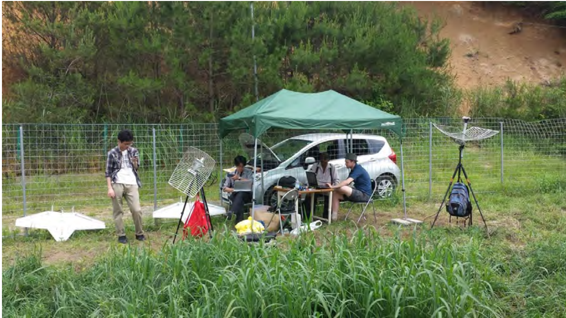
Figure 3: DataHawk Flock used in the June, 2015 campaign in approved airspace at Shigaraki, Japan, comparing radar returns with in-situ DataHawk measurements. Two of the five DataHawks from this campaign are visible in the picture (white planes, left), with equipment from one DataHawk Flock pod. An average of 3 flights per day were conducted over a 10 day period. The pod and batteries were shipped separately by commercial air cargo.
