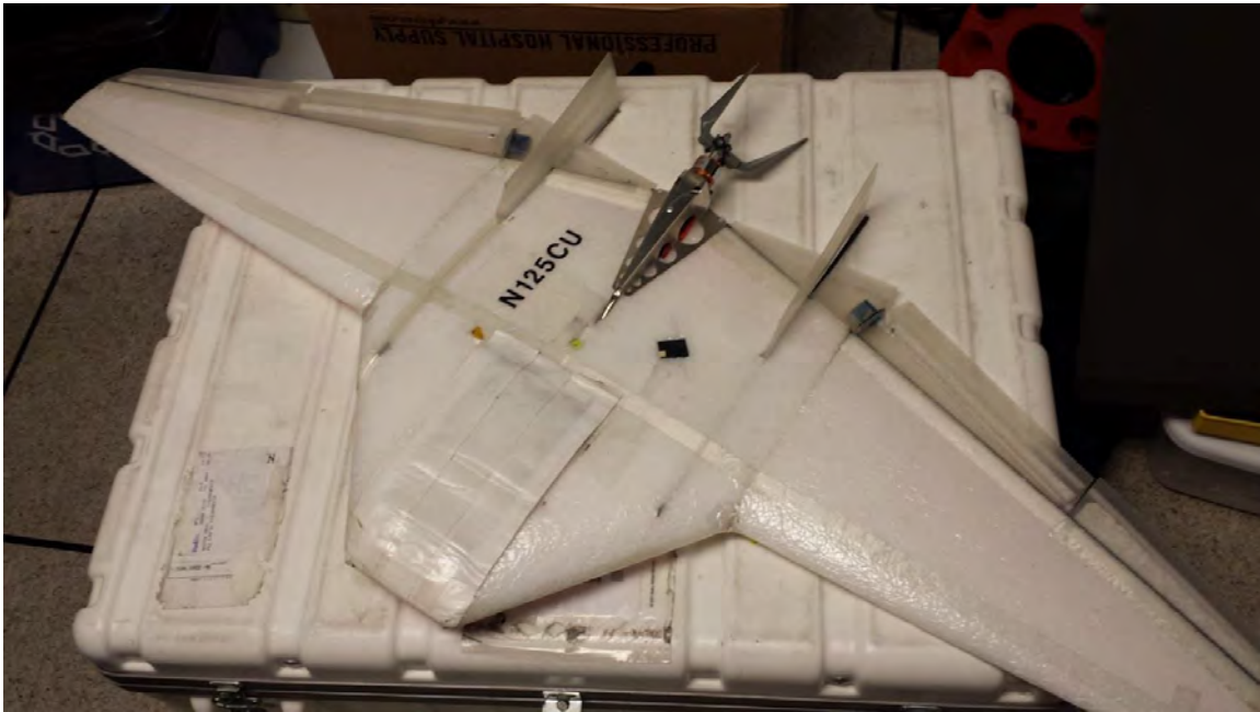
Figure 1: Assembled DataHawk 2 aircraft, shown on top of the DataHawk Flock Pod shipping case. Wing span is 52in., gross weight is 1.1Kg, flight speed ranges between 12 and 24 m/s, and duration in level flight is about 100 minutes.
