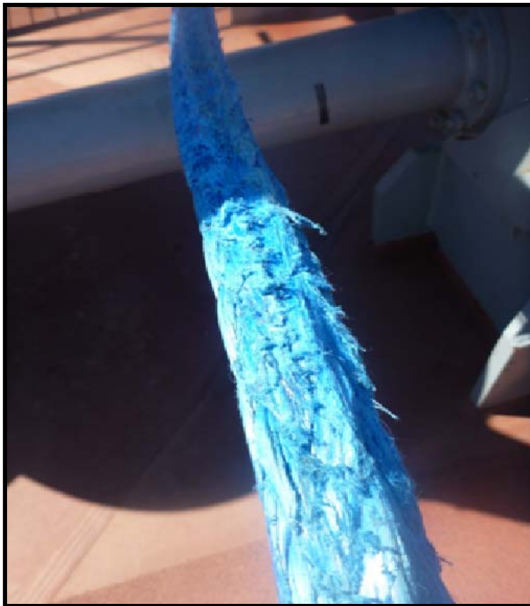
Figure 4-2. Mooring Line Damage
