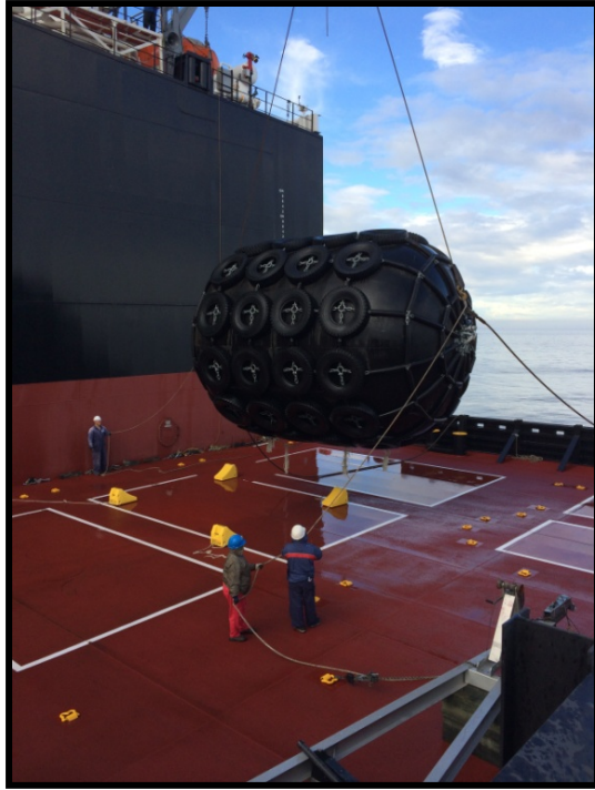
Figure 1-3. Crew Members Positioning Fenders
