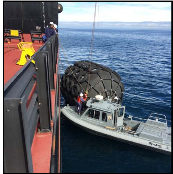
Figure 1-3. Crew Members Positioning Fenders
