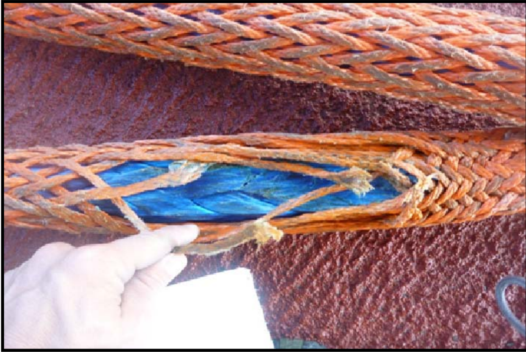
Figure 4-3. Mooring Line Damage
