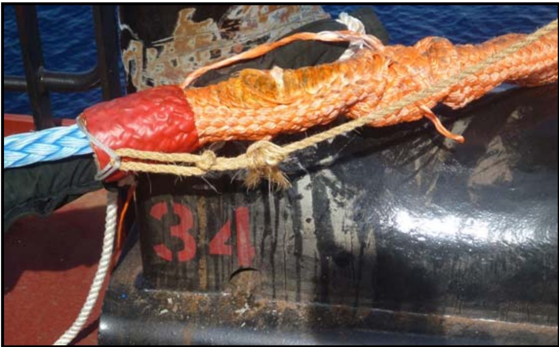
Figure 4-4. Mooring Line Damage
