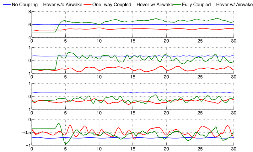
Figure 5 - Attitude response of the simulated helicopter hovering over the SFS2 flight deck.
