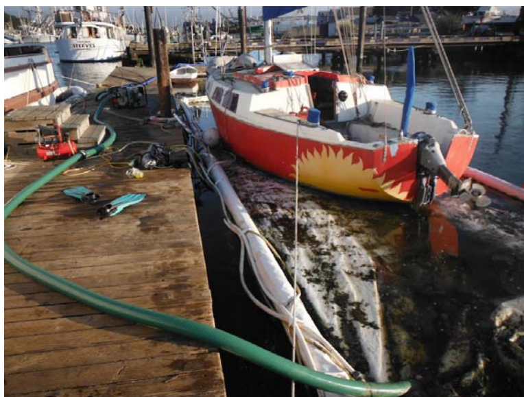
Figure 6. Hull cleaning effluent being vacuumed from within an Innermost Containment Systems barrier.
