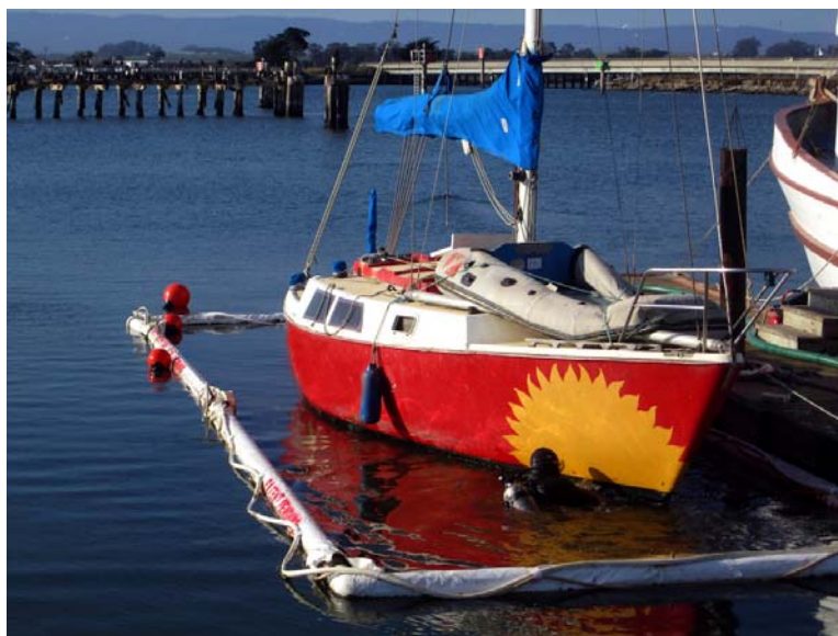
Figure 5. Vessel undergoing hull cleaning within Innermost Containment Systems barrier.
