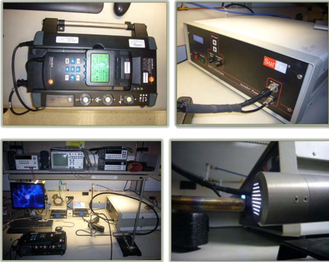
Figure . Setup a 13.56 MHz radio frequency dielectric barrier plasma system
