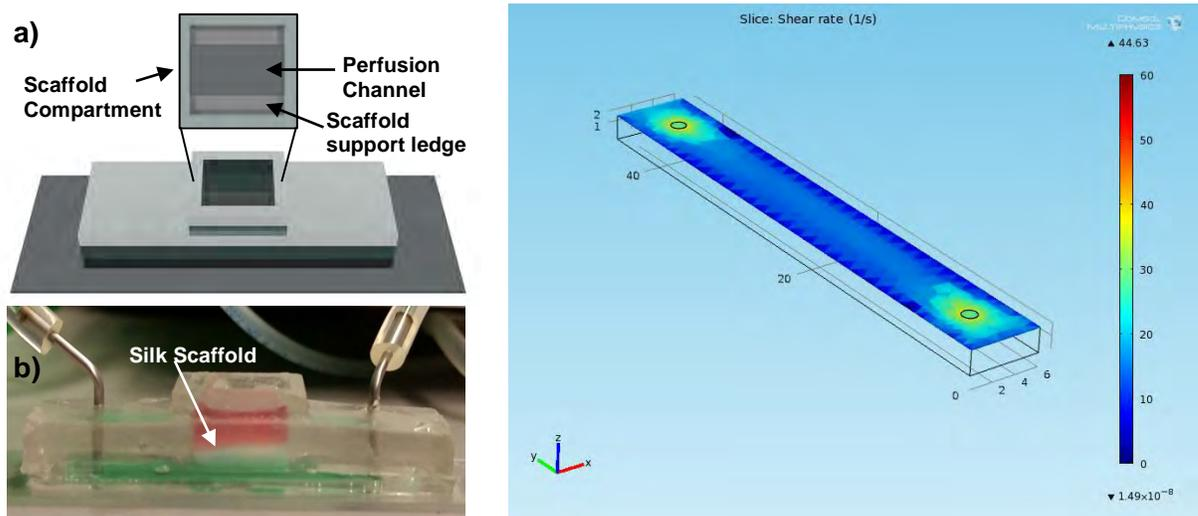
**Figure 1** (a) AutoCAD model of the 3D perfusion bioreactor. The silk scaffold dimensions are several millimeters wider than the channel dimensions to allow for stable scaffold incorporation. (b) Photograph of the final assembled PDMS bioreactor. (c) COMSOL model of shear rate at the height of the scaffold within the channel.
