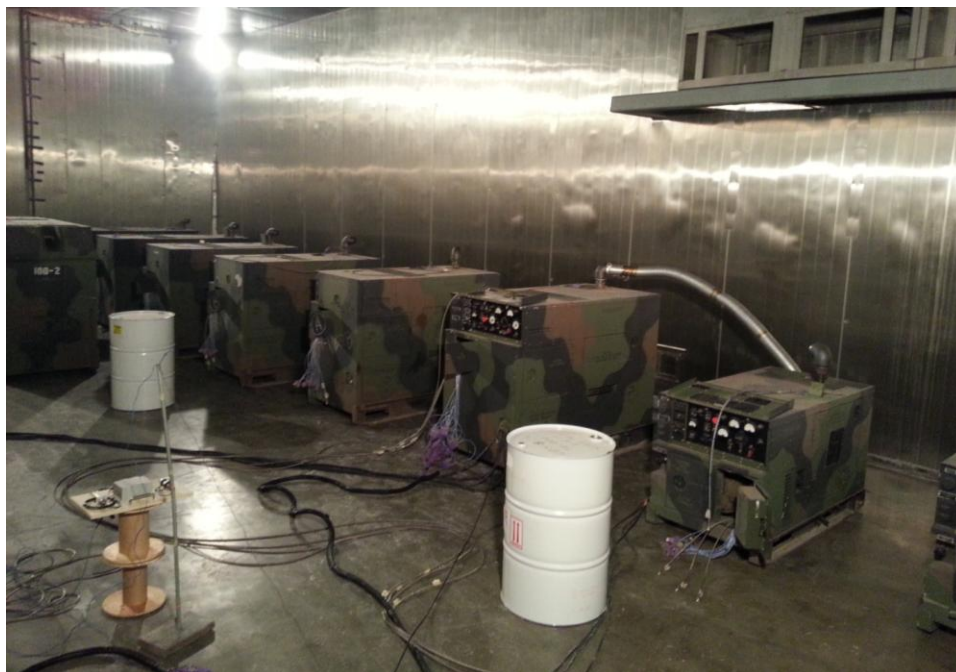
Figure 1. 15kW Generator Ready for Environmental Testing – Others on Standby
