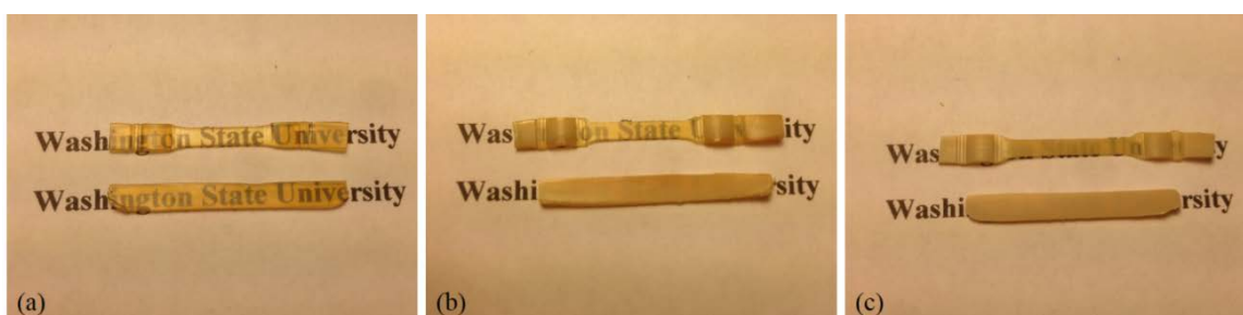
Figure 6.9 Photos of the LCEs after the static tensile tests: (a) BP-SA-05, (b) BP-SA-07, and (c) BP-SA-10.
