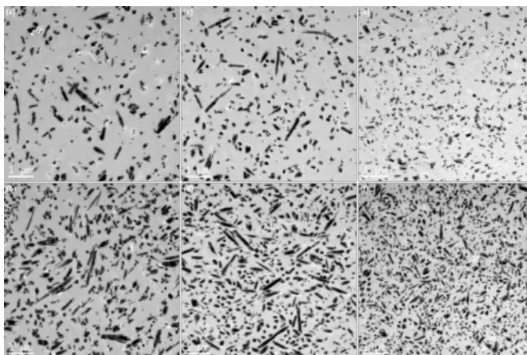
Figure 3.2 TEM images of \text{ZrW}_2\text{O}_8 /Epoxy nanocomposites with different types and volume fractions of nanoparticles: (a) 10 vol. % Type-1 \text{ZrW}_2\text{O}_8 , (b) 20 vol. % Type-1 \text{ZrW}_2\text{O}_8 , (c) 10 vol. % Type-2 \text{ZrW}_2\text{O}_8 , (d) 20 vol. % Type-2 \text{ZrW}_2\text{O}_8 , (e) 10 vol. % Type-3 \text{ZrW}_2\text{O}_8 , (f) 20 vol. % Type-3 \text{ZrW}_2\text{O}_8 .
