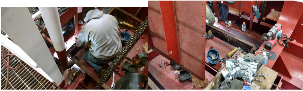
Stuffing tubes being welded in on 3.5 khz sub-bottom profiler. Cable penetrations in side of enclosure will allow lifting the lid off to service individual transducers.
