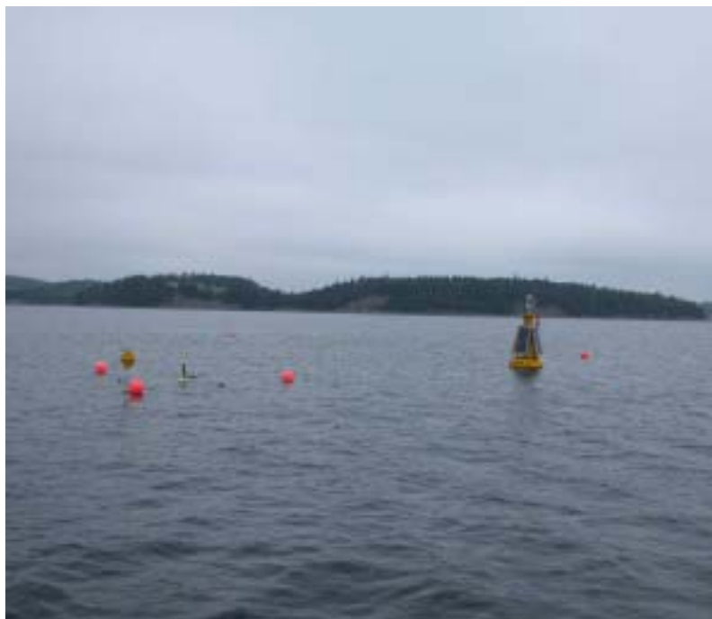
Figure 2. The Optical Buoy Array as deployed in Lunenburg Harbour. The primary buoy contains physical and meteorological instruments, as well as power and communication subsystems; the secondary smaller buoy contains the optical instrumentation.
