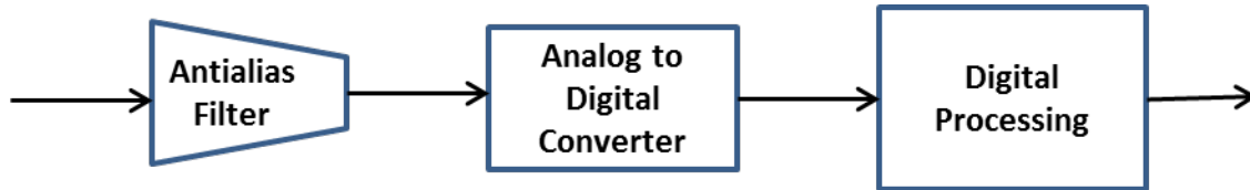
Figure 1. Typical anti-aliasing filter used in digital signal processing (Ref 1).
