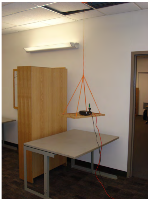
Figure 9: The receiver sits on a wooden platform which hangs from the ceiling. The platform is equipped to swing parallel to the wall through 0.20 m.
