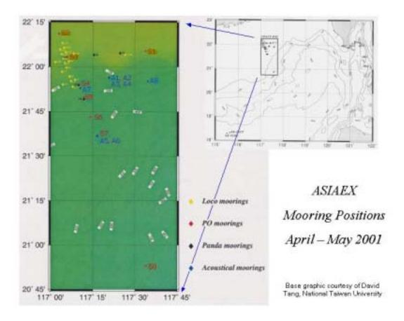
Figure 1. Location of the WHOI/NPS/NTU moored array deployed in the South China Sea during the ASIAEX experiment, April to May 2001. The red diamonds numbered S1 – S8 are the physical oceanography moorings and the blue diamonds numbers A1 – A8 are the acoustics moorings. The Low-cost (LOCO) moorings are indicated in yellow and the PANDA moorings in black.
