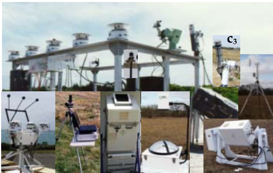
Figure 1. The SMART system: (a) many shortwave and longwave broadband radiometers, (b) shadow-band radiometer, (c) sun photometers, (d) solar spectrometers, (e) micro-pulse lidar, (f) whole-sky camera, and (g) microwave radiometer, as well as (h) meteorological probes for atmospheric pressure, temperature, humidity, wind speed/direction and (k) surface moisture content.
