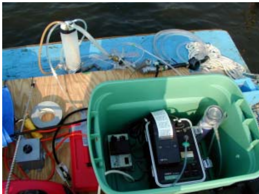
Figure 1. Photograph of the continuous radon-in water monitor. [The exchanger, upper left, mixes seawater from a submersible pump with a stream of air that is then routed to the radon monitor, lower right]
