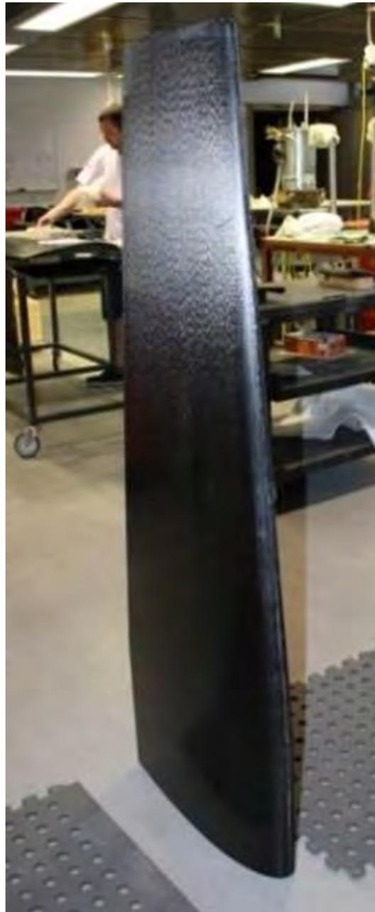
*Figure 4: Completed Carbon/fibreglass composite hydrofoil prior to instrumentation.*
