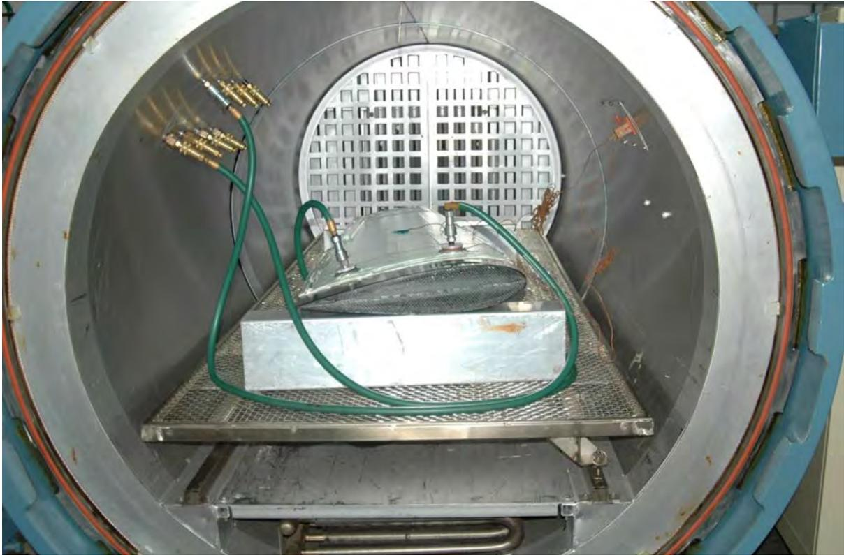
Figure 13: Hydrofoil in autoclave oven prior to curing.
