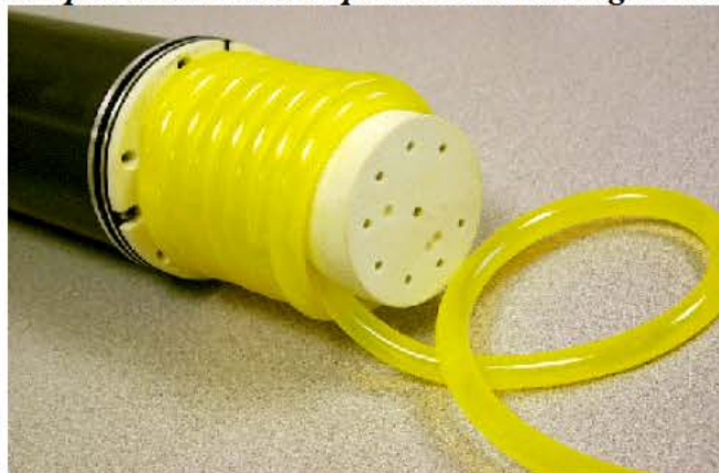
Fig. 4. Acid storage section. The acid is stored within the yellow tube. One end of the tube is fed from the aluminum tube, the other feeds into the melter section. The acid is delivered to the melter section when the pump first starts.
