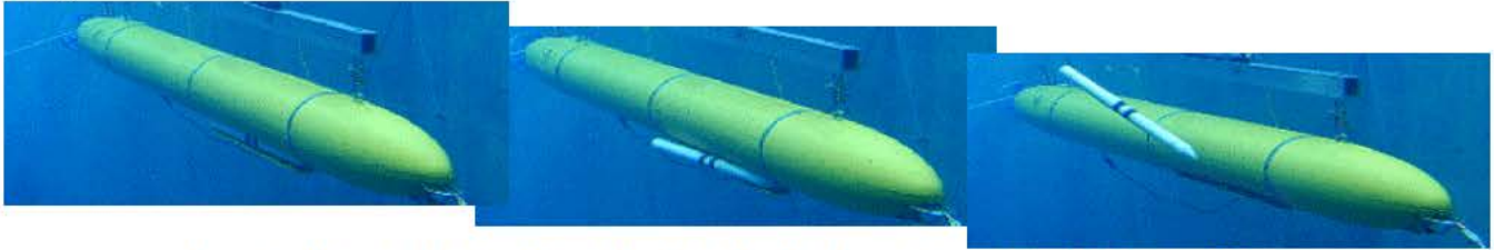
Fig. 7. These pictures show the launch of a buoy from the ALTEX vehicle.
