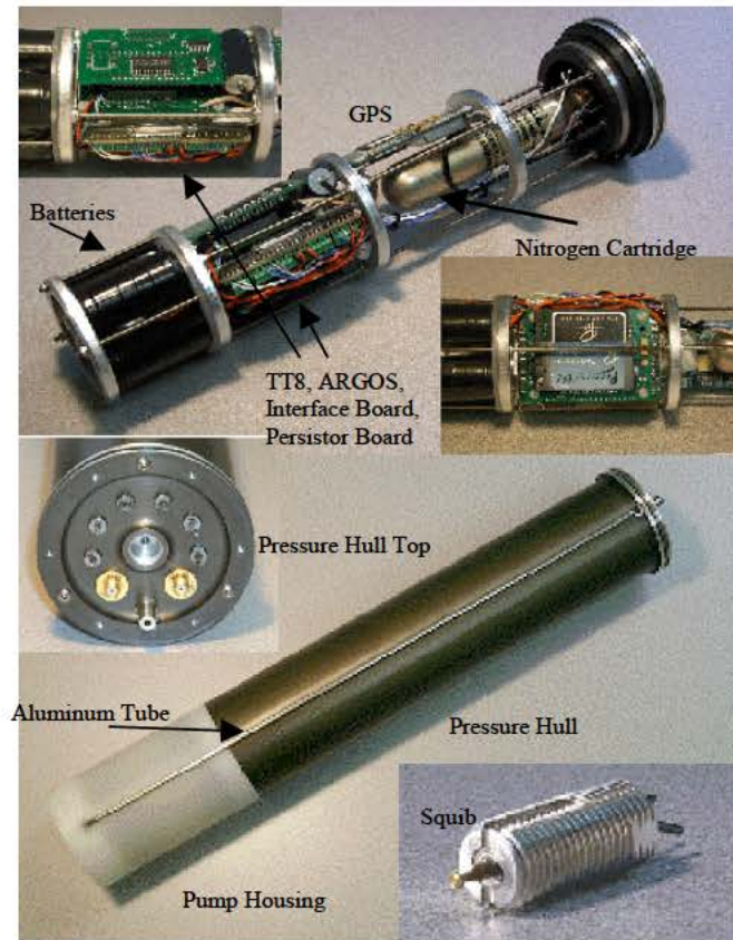
Fig. 3. Pump housing and pressure hull section. Also shown are the cage and electronics inside the pressure hull, the top of the pressure hull showing the feedthroughs, and the squib device used to puncture the nitrogen cartridge.
