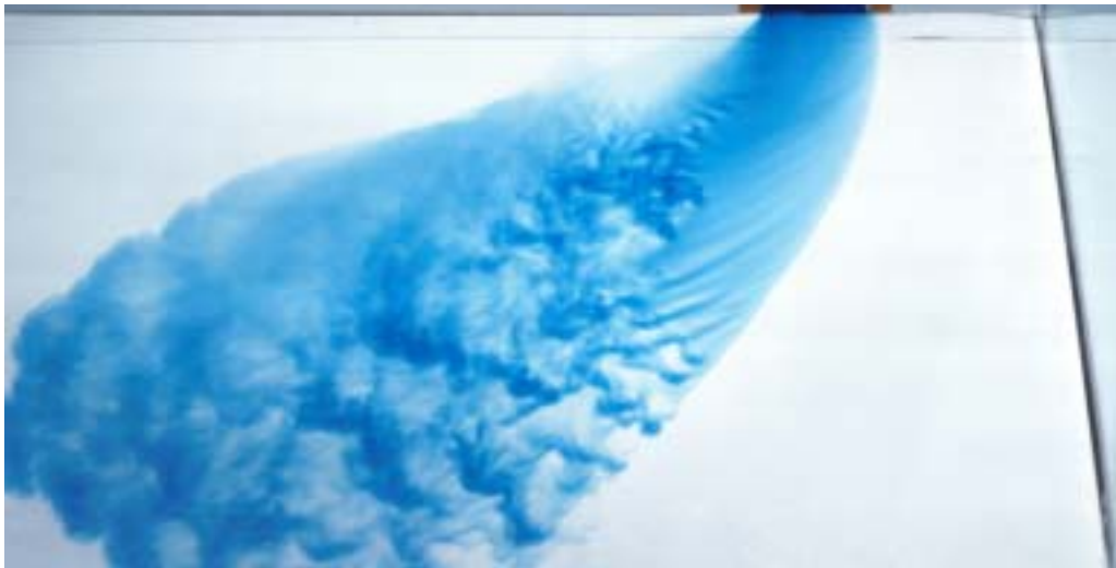
Figure 1. Side view photograph of a plume of dyed salty water sinking downward above a sloping bottom in transparent, fresh rotating water. The intersection of the sloping bottom with a vertical side of the co-rotating rectangular tank is visible on the right. The plume curves toward the right in the direction of flow, but it bends toward the left with depth in this picture as the flow is directed toward the camera. Waves and small-scale turbulence are visible. Also near the source is a patch of mixing that is associated with cyclonic gyre formation in the clear water. The cyclonic gyre typically lifts a lens of blue fluid and moves it to the left with uniform sideways velocity.
