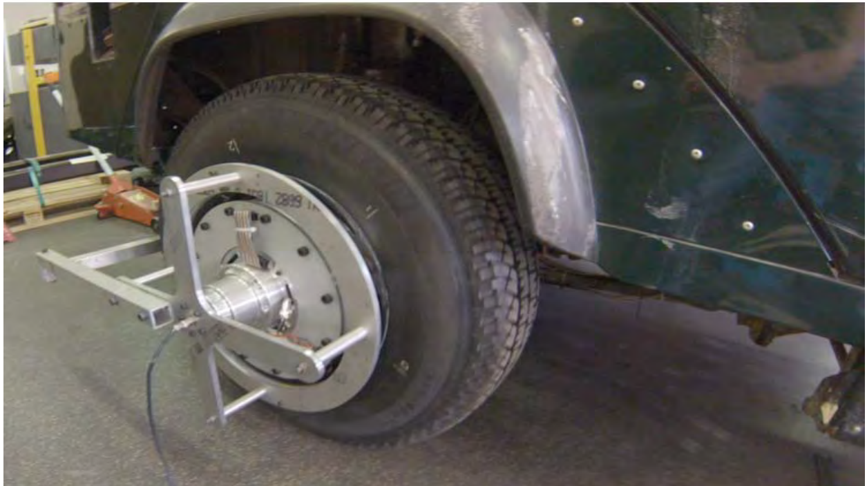
Figure 6 – Complete T2-CAM system with VDG wheel force transducer fitted to test vehicle
