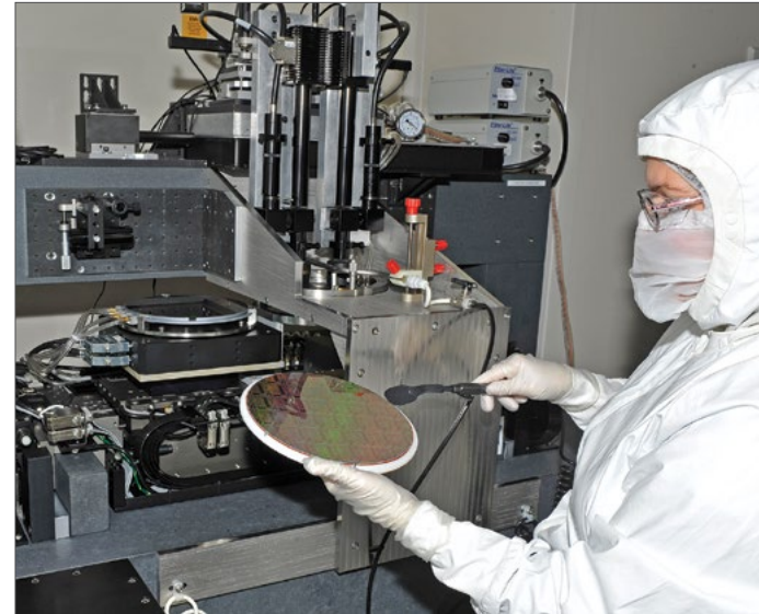
Donna-Ruth Yost of the Quantum Information and Integrated Nanosystems Group prepares for a wafer-scale bonding of 8-inch-diameter optical photonic and complementary metal-oxide semiconductor (CMOS) wafers.
