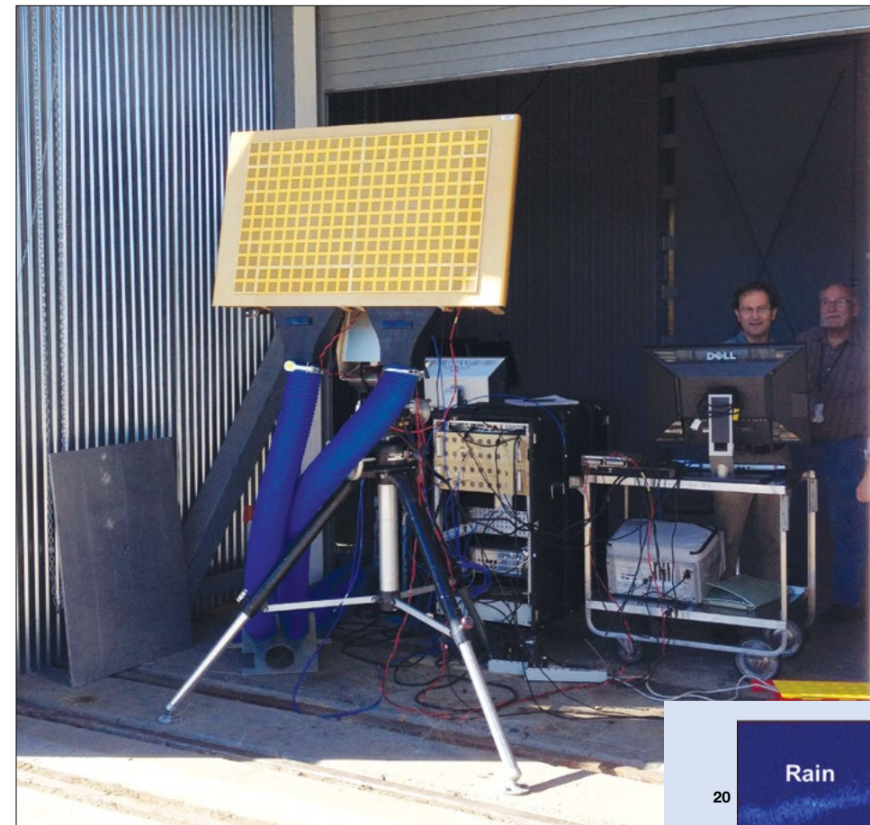
The two-panel prototype MPAR array (left) is used at Hanscom Field to collect observations of aircraft and weather in the vicinity. The range-Doppler plot below is of the weather and aircraft observed by this prototype array.
