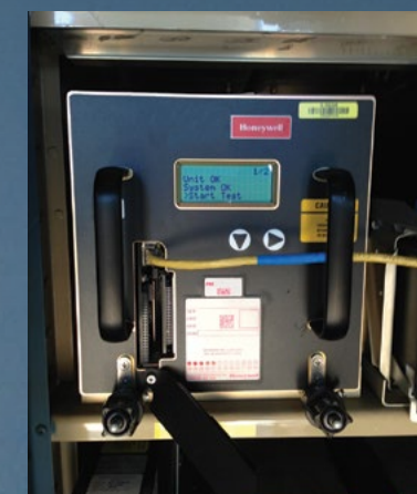
ACAS X logic is implemented in the Honeywell International Inc. prototype used in the 2013 proof-of-concept flight test.
