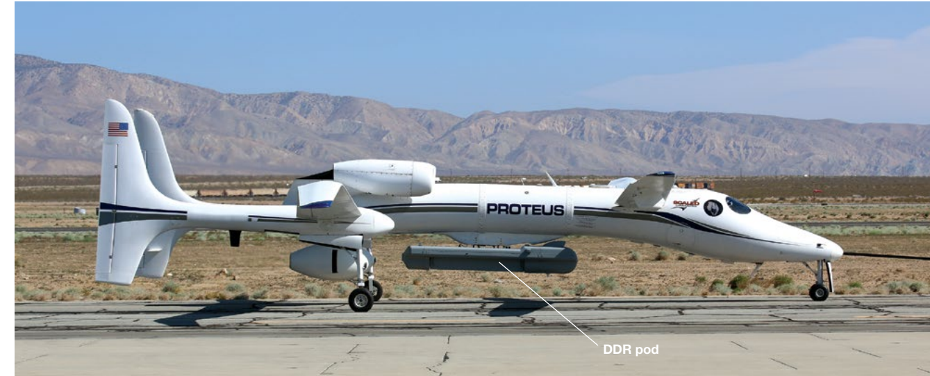
Lincoln Laboratory helped to define an open-systems architecture and supported the development of advanced algorithms for the U.S. Air Force's Dismount Detection Radar (DDR) prototype. The DDR pod was integrated onto a Scaled Composites' Proteus aircraft and underwent development testing at the Mojave Air and Space Port and Edwards Air Force Base in Southern California.
