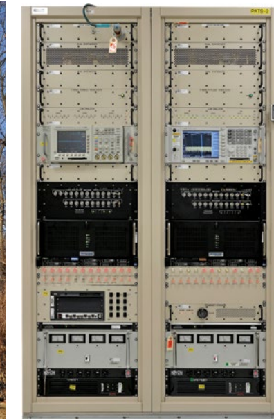
The Over-the-Air Ka-band Test Terminal (far left) and the Protected Tactical System Advanced Test Set (left) will be utilized together to test the new Protected Tactical Waveform. The Lincoln Laboratory-built implementation of the waveform will be used in lab and over-the-air tests to validate the capabilities of vendor implementations of the waveform.
