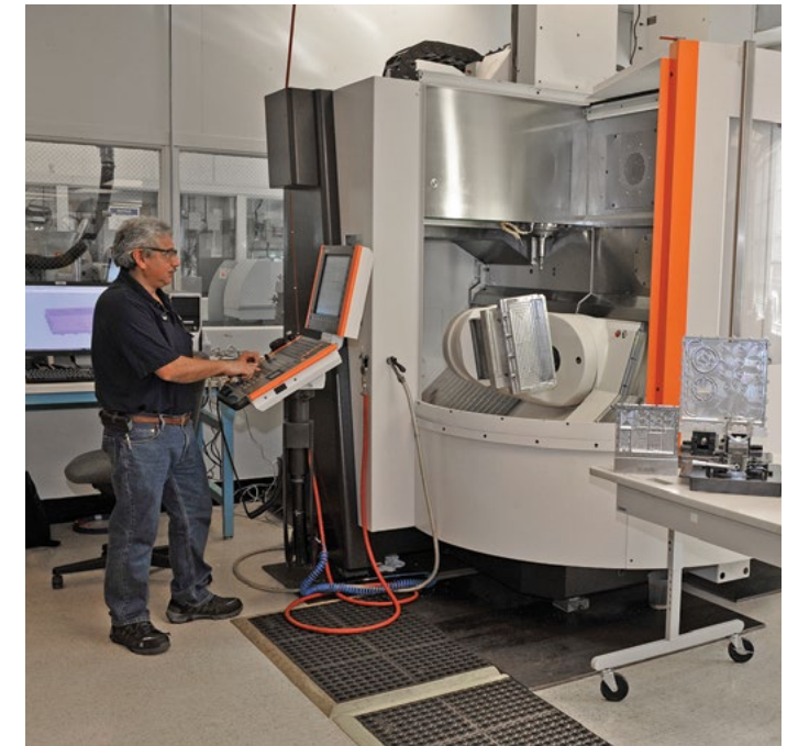
The five-axis machining equipment rapidly and efficiently produces components for prototype systems, resulting in savings in energy, manpower, and time.
