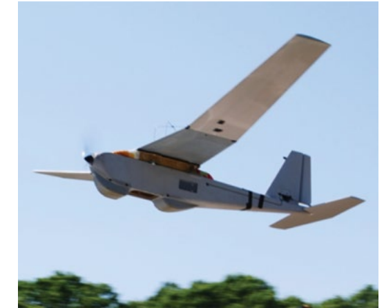
This Puma unmanned aerial vehicle is equipped with the vector sensor that the Laboratory developed to provide a tactical geolocation capability. The Puma's first flight occurred at the Camp Edwards air field in Massachusetts.
