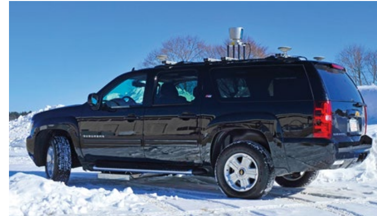
The Laboratory's new ground vehicle test bed is supporting current and future unmanned autonomous systems work in localization, perception, and mapping. A novel Lincoln Laboratory-designed localizing ground-penetrating radar positioned underneath the vehicle enables 3-centimeter-level real-time localization to a prior map at travel speeds up to 60 mph. A lidar mapping sensor, camera, and dual differential global positioning systems were also integrated into the mobile test bed to provide accurate mapping and localization capabilities.
