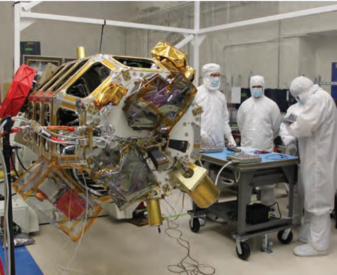
Researchers in the Optical Communications Technology Group prepare to verify electrical interconnections prior to powered testing of the Lunar Laser Communication Demonstration terminal that is integrated onto the spacecraft.
