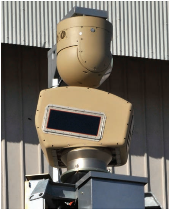
WISP-360 has a ruggedized housing that is sealed against dust, moisture, and humidity. The window in the casing is made of germanium and has a scratch-resistant carbon exterior coating.
