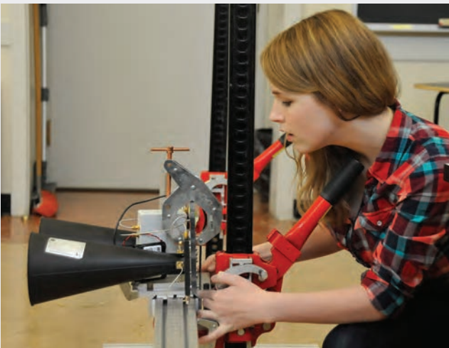
A new IAP course proffered a challenge: Find a Needle in a Haystack with 3D Imaging Radar. Participants set up an ultrawideband imaging radar that they used to image a haystack in which needles, skewered into Styrofoam balls, had been hidden. The onscreen image of the haystack (below) reveals the location of needles buried inside the hay. This two-day workshop built upon techniques covered in the other two radar-building IAP courses led by Lincoln Laboratory technical staff.
