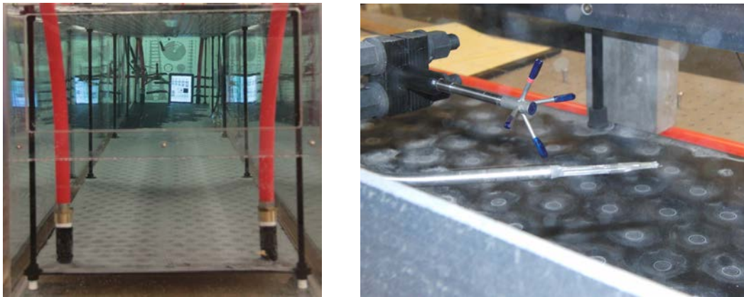
Figure 1. Laboratory tank at NRLSSC. The photo on the right shows the Vectrino profiler ADV and the CT temperature probe.
