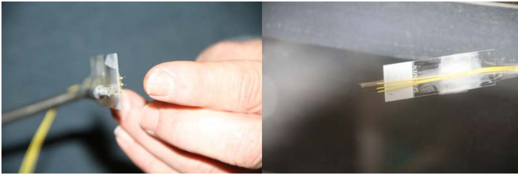
Figure 7. Fiber optics sensors next to PME microstructure temperature sensor (FP07) in the tank.
