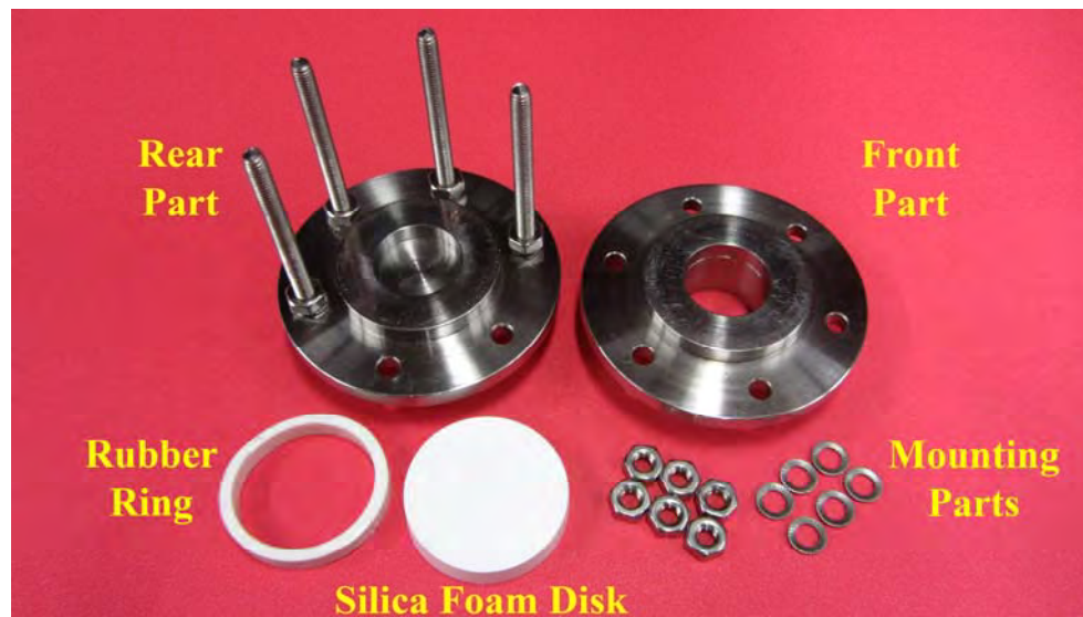
Fig. 3.2 The shear promotion holder and a silica foam disk sample.
