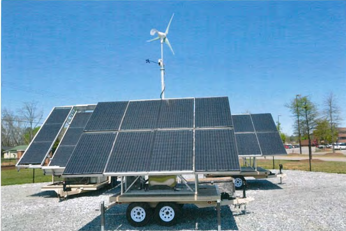
Figure 1. Mobile Solar Units at Fort Valley State University (L-R) Mohave 3 solar array, Alvord Drone with Air Dolphin wind turbine, Alvord solar array
