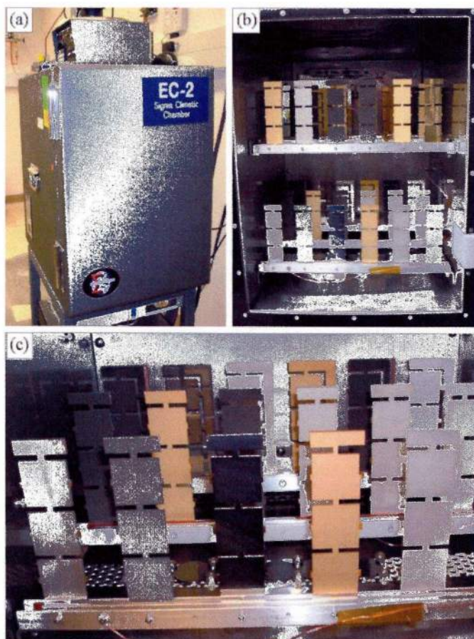
Figure 3-8. (a) Digital image of the thermal cycle chamber used (EC-2 Sigma Climatic Chamber), (b) Digital image of coupons mounted in TC chamber for aging, and (c) Close-up view of samples in TC chamber.
