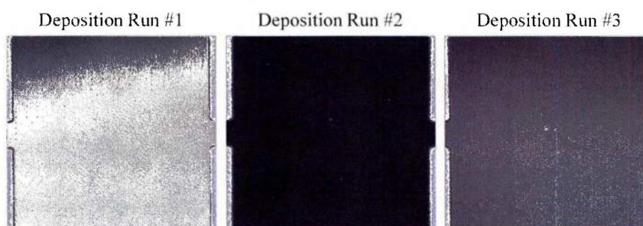
Figure 4-3. Optical images of Group 1 Ni sputtered copper samples showing the visual variations in the appearance of the coating based on the deposition run: Run #1 (left), Run #2 (middle), Run #3 (right).
