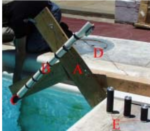
Figure 1. Equipment used. A denotes drop angle device, B mine injector, C infrared light sensor, D output to universal counter, E mine shapes.
