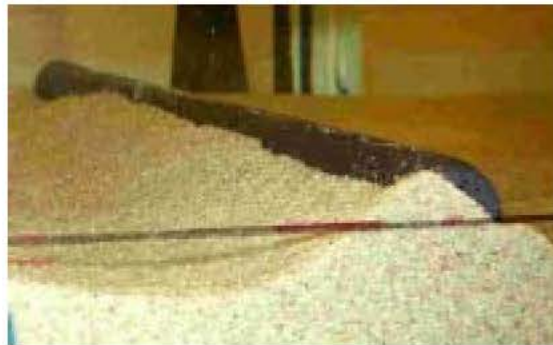
Figure 5. Sand accumulation along a mine at relatively small values of \Psi ( = 4 , KC = 20 , Re = 6300 ).
