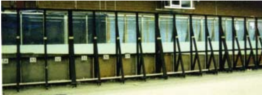
Figure. 1. A side view photograph showing various features of the experimental wave tank (32 x 0.9 x 1.8 m). The distance between vertical bars is 61 cm.
