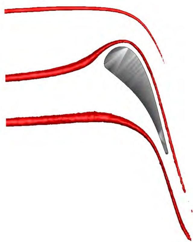
Figure 5.5: Isosurfaces of 20% normalized concentration (concentration is normalized with respect to inlet concentration). The suction side hot streak is acquired from the low concentration data set, while the center and pressure side hot streaks are acquired from the high concentration data set.
