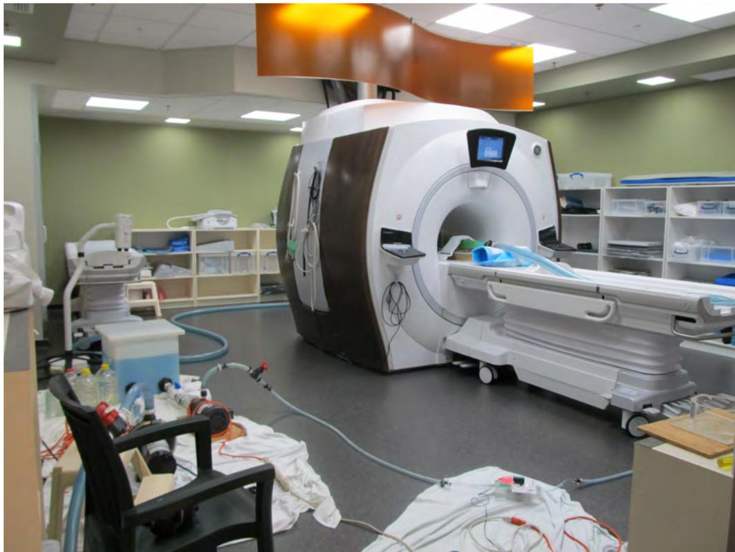
Figure 3.10: 3T1 Magnet Suite at Richard M. Lucas Center for Imaging, Stanford University. The test channel is inside the transmit-receive head coil inside the bore of the magnet. A 25 gallon tank full of 0.06M copper sulfate solution completes a closed loop system of pumps, valves, and flowmeters to recirculate the working fluid for an MRV scan.
