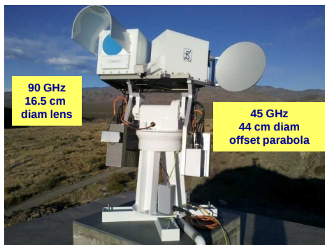
45 and 90 GHz solar polarimeters POEMAS
