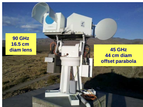
45 and 90 GHz solar polarimeters POEMAS
