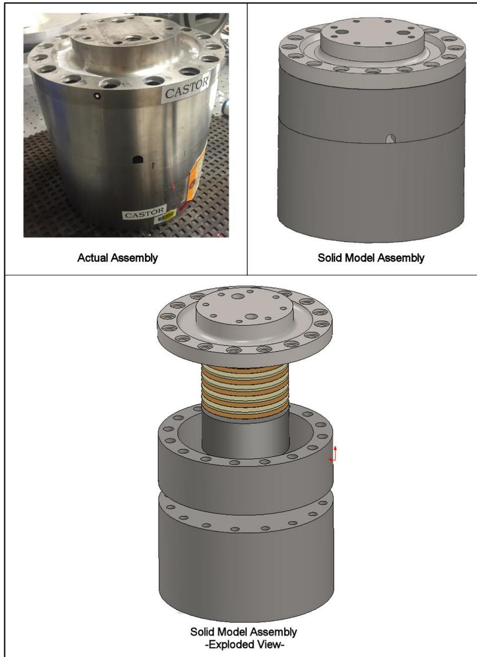
Figure 23. Piezoelectric Shaker Table System Solid Model
