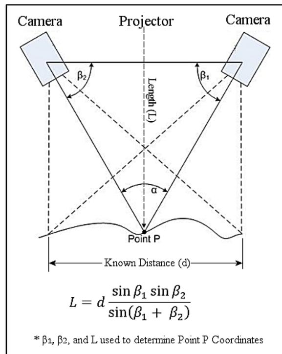
Figure 6. 3D Scanner Triangulation of a Point (Rhoades, 2011:30)
