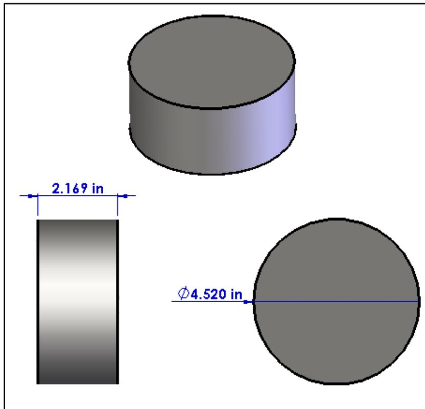
Figure 41. Piezoelectric Shaker Table Spacer Component Dimensions
