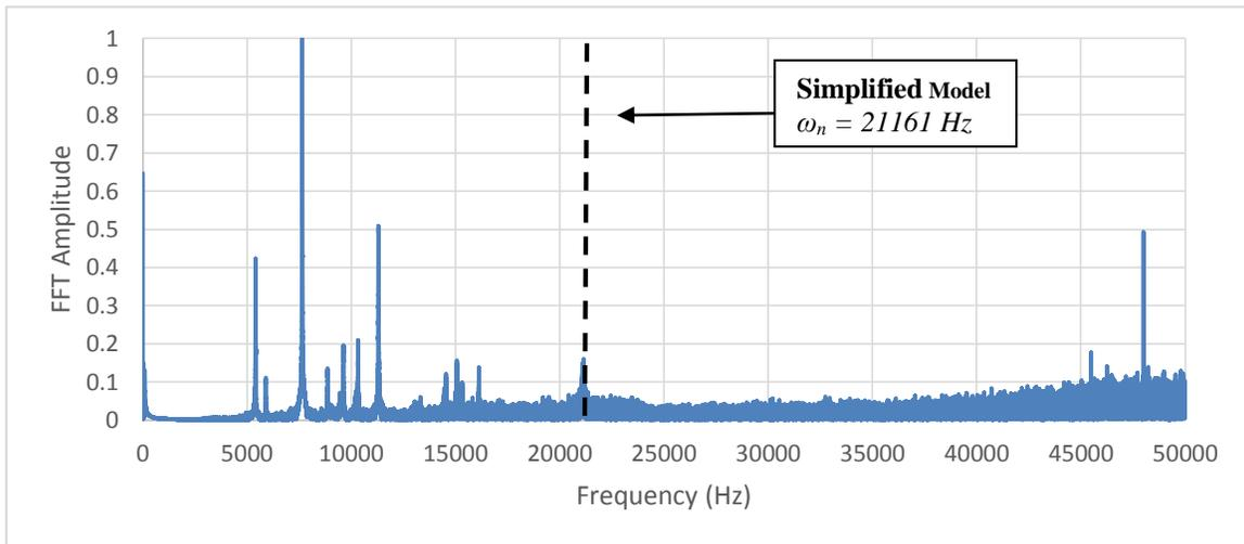
Figure 31. Piezoelectric Shaker Table Ping Test Response
