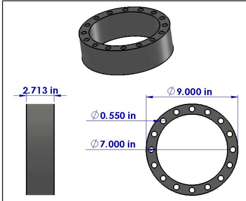
Figure 40. Piezoelectric Shaker Table Collar Component Dimensions
