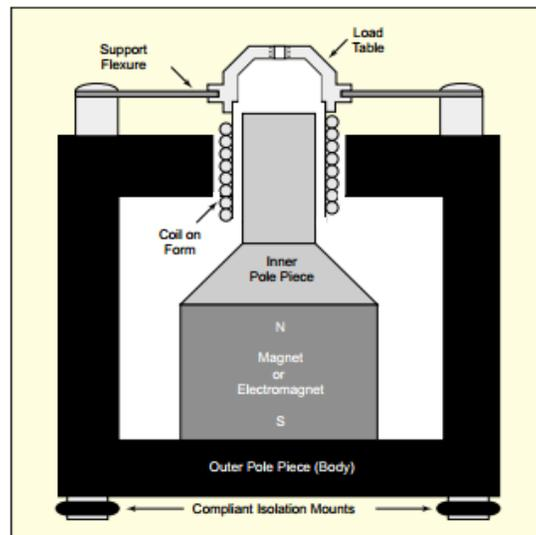
Figure 1. Electrodynamic Shaker Structure (Lang and Snyder, 2001:2)
