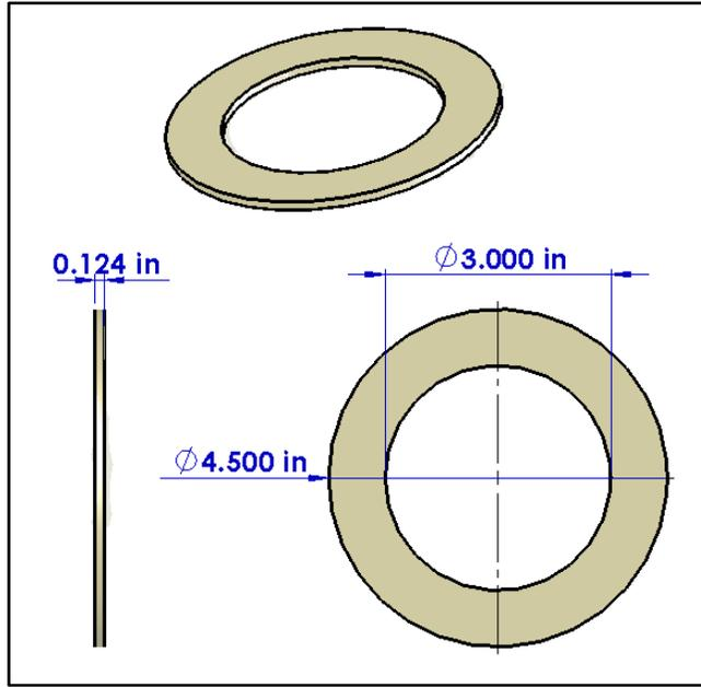
Figure 43. Piezoelectric Shaker Table Crystal Component Dimensions
