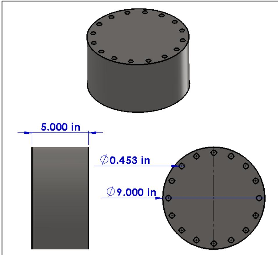
Figure 39. Piezoelectric Shaker Table Base Component Dimensions
