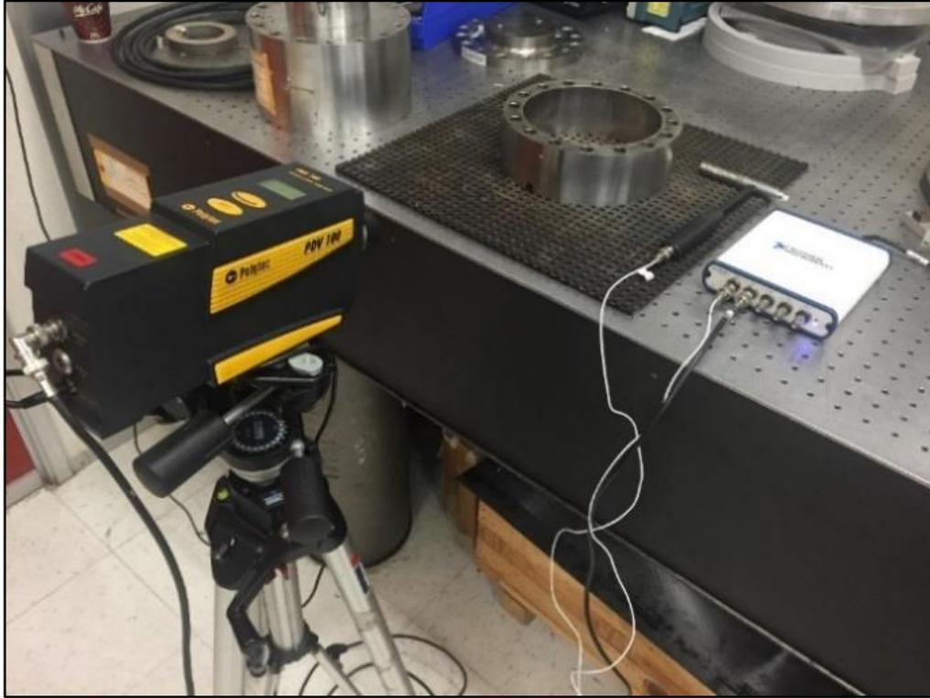
Figure 21. Ping Test Experimental Setup
