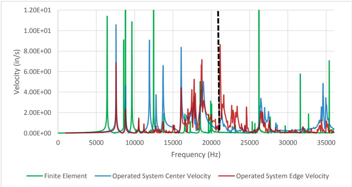
Figure 36. Finite Element and Physical System Response Comparison
