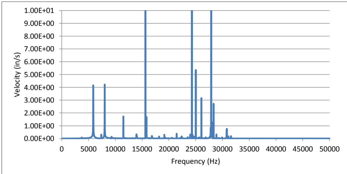
Figure 38. Finite Element Response Using Maximum Surface Velocity
