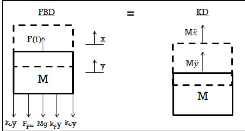
Figure 12. Simplified Piezoelectric Shaker Table FBD and KD
