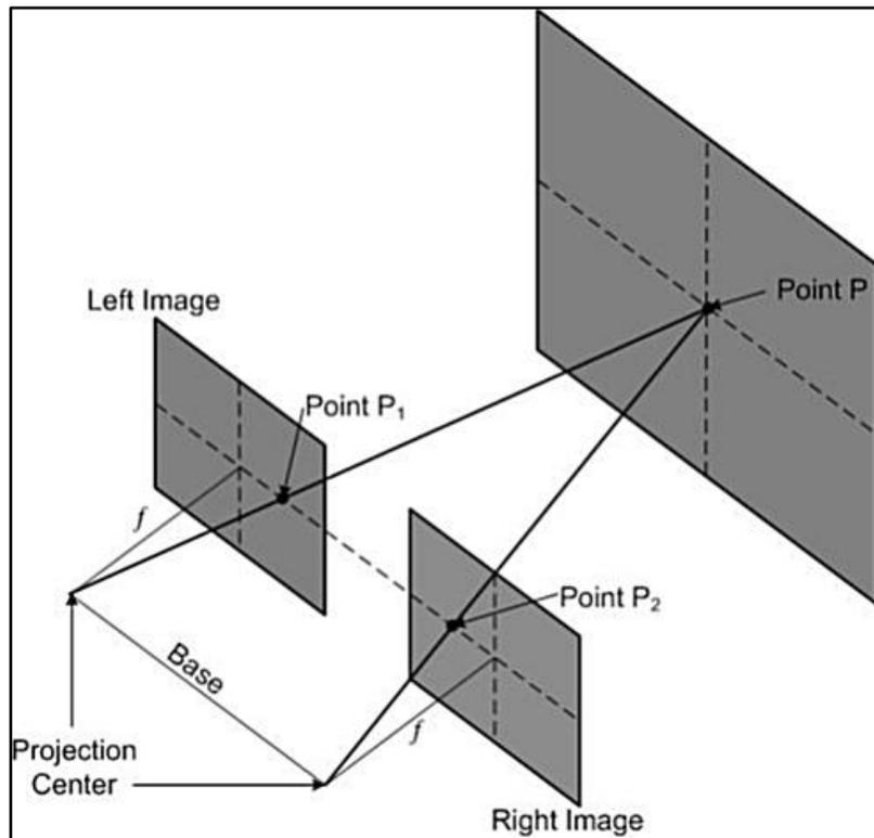
Figure 7. Photogrammetry Center of Projection (Rhoades, 2011:25)
