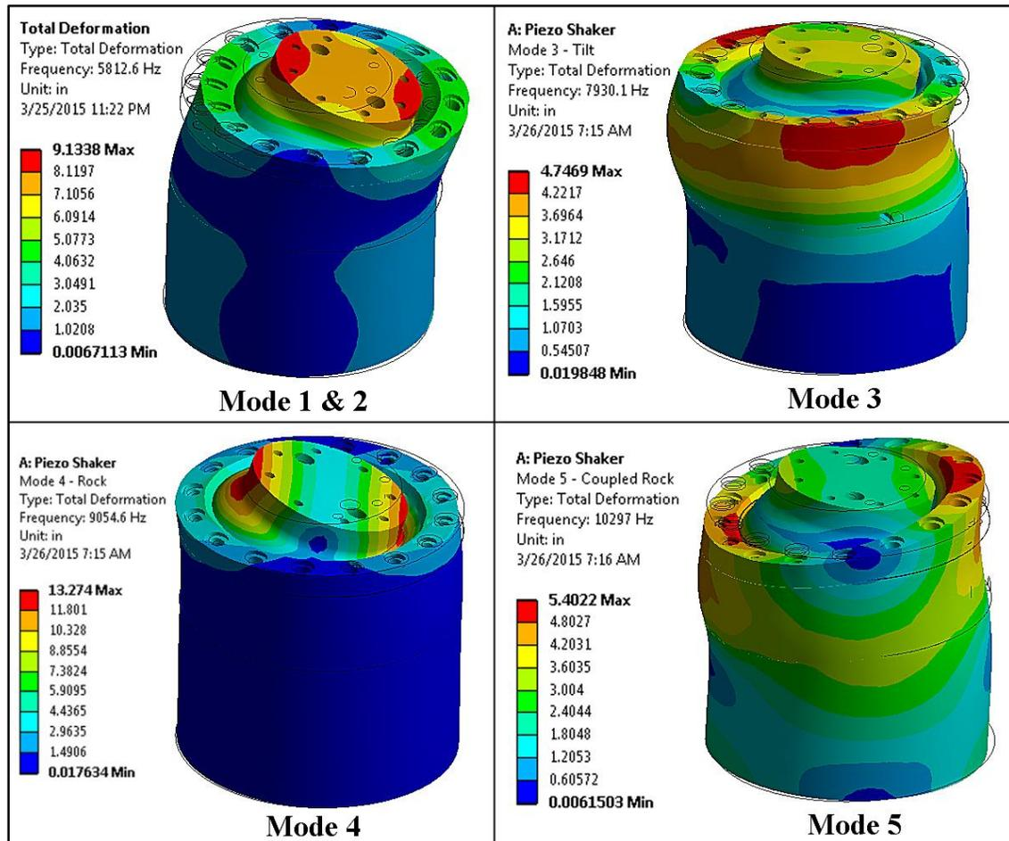
Figure 32. First Five Piezoelectric Shaker Modes
