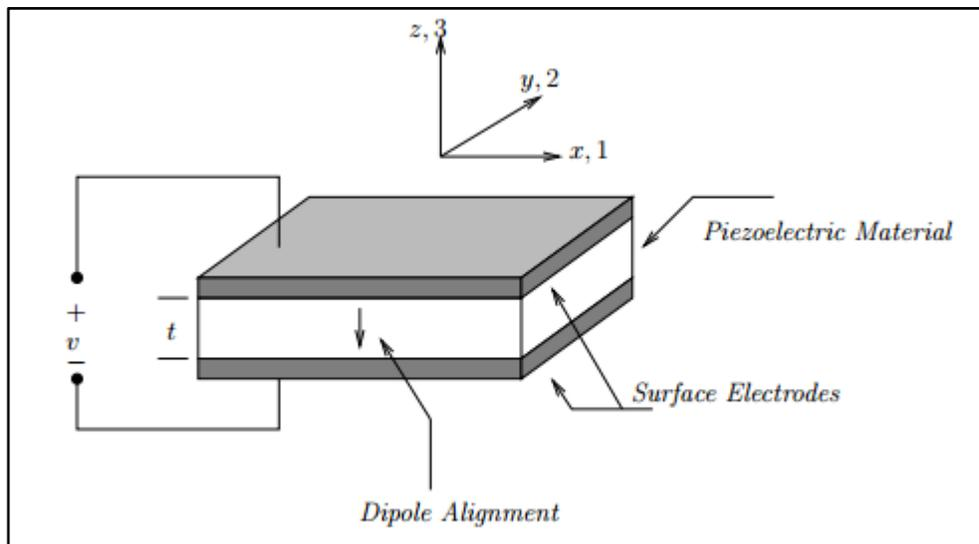
Figure 4. Piezoelectric Stack Electrical Circuit (Moheimani and Fleming, 2006:14)
