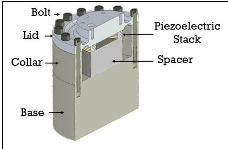
Figure 3. Piezoelectric Shaker Cross Section
