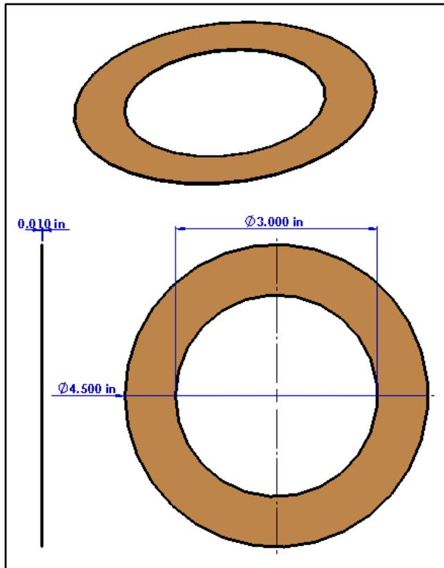
Figure 44. Piezoelectric Shaker Table Electrode Component Dimensions
