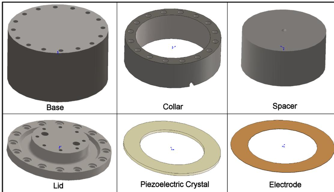
Figure 16. Piezoelectric Shaker Table Component Solid Models
