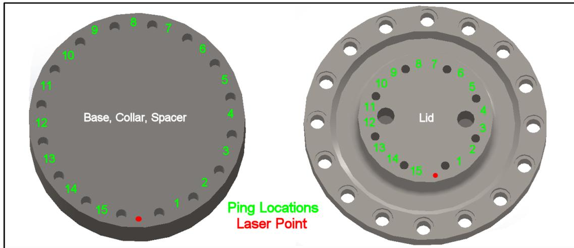
Figure 22. Component Ping and Laser Measurement Locations
