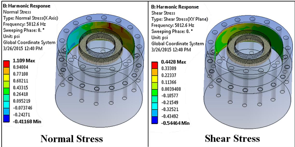
Figure 34. Free Surface Normal and Shear Stress
