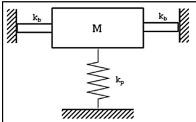
Figure 11. Simplified Piezoelectric Shaker Table Mechanical Model
