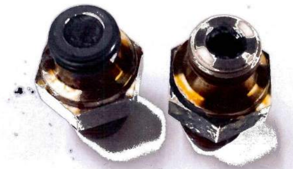
Figure 46 Coke formation in heating hose fittings
