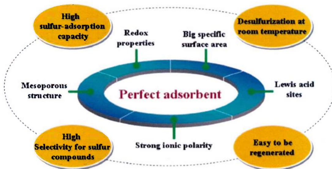
Figure 1. Ideal adsorbent model for desulfurization of Jet-A fuel
