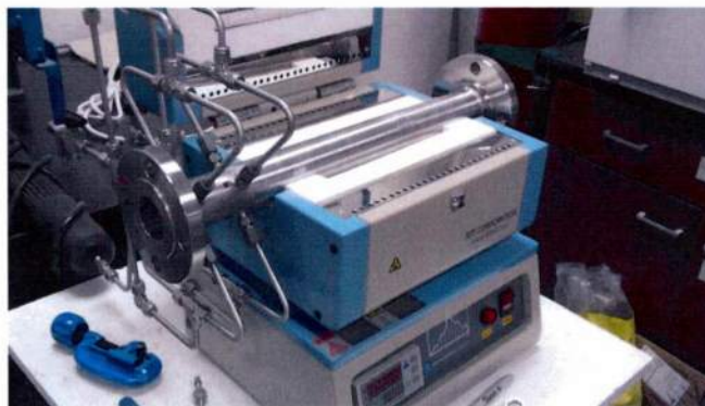
Figure 36 ATR reactor with steam and air distribution tubing
