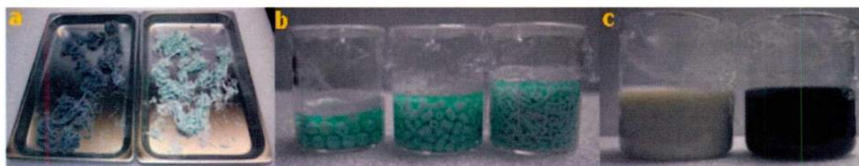
Figure 2 Ni-Ce/Al 2 O 3 -SiO 2 adsorbents prepared by three different methods. (a) Extrusion molding—the best method adopted; (b) wet impregnation; (c) sol-gel.
