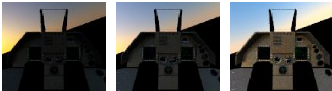
Figure 12: Illustrations of the effect of ambient illumination (shortly after dawn) on the interior of the cockpit as the heading direction is changed. On the left, the model is aimed just to the right of the rising sun, in the middle the sun is further to the left, and on the right the heading is directly away from the sun
