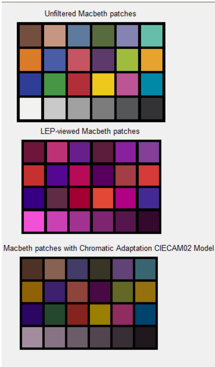
Figure 23: Example of the effects of chromatic adaptation on color appearance of the MCC viewed through a colored filter with a pink tint
