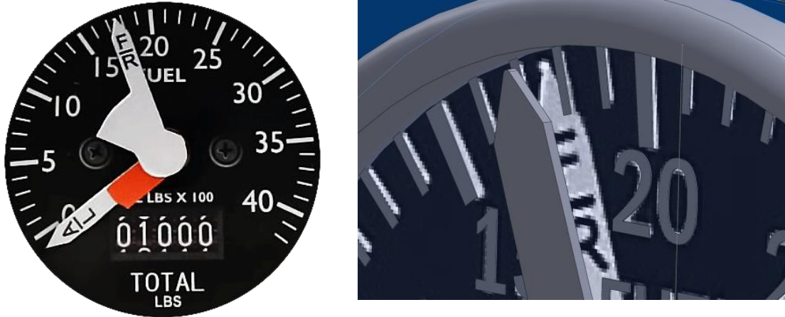
Figure 8: Example of a reflective component (fuel gauge) that was modeled in SolidWorks. On the left is the original bitmap image (photograph) of the gauge and on the right is a closeup example of the SolidWorks geometry built on top of the bitmap
