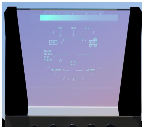
Figure 10: Simulation of the HUD without a filter in the field of view under daytime ambient lighting
