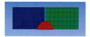
Smoothed-particle hydrodynamics (SPH) is applied for all parts. The SPH particle size is .4 mm, with the assumption that modeling dust smaller than .4 mm can be ignored. A stationary boundary is applied on the edges. The two tiles SiC and SiC 2 are identical with the same dimensions and properties. They are utilized as different materials to differentiate the damage on each tile. The gap size will be changed for different simulations.
