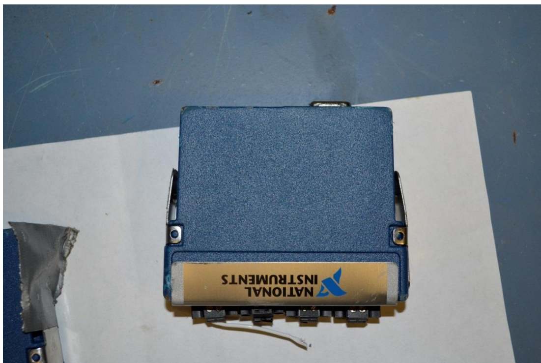
FIGURE A-7. Damaged c-Module, 2nd Slot.
