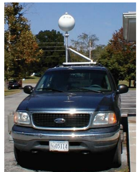
Fig. 4. ET probe mounted on vehicle for testing.
