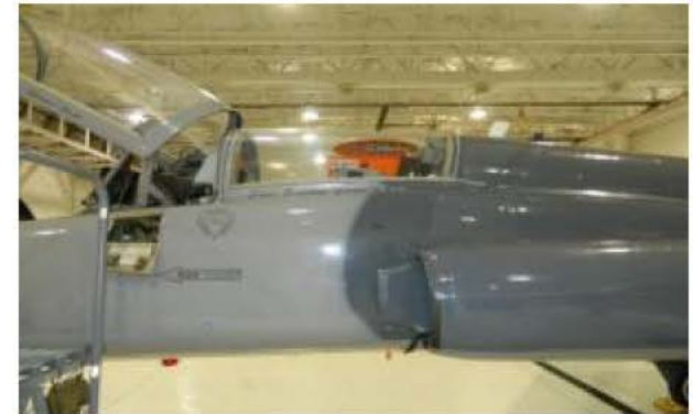
A Rear Cockpit Pallet mounted in the back of a T-38 Talon
