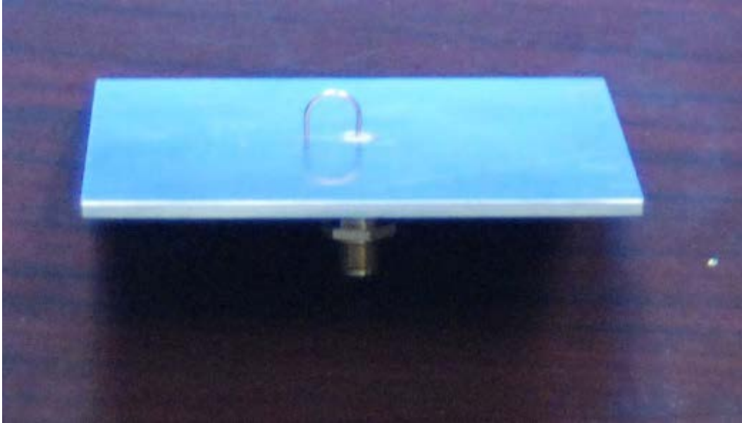
Fig. 5 Standard SMA connected half loop receiver
