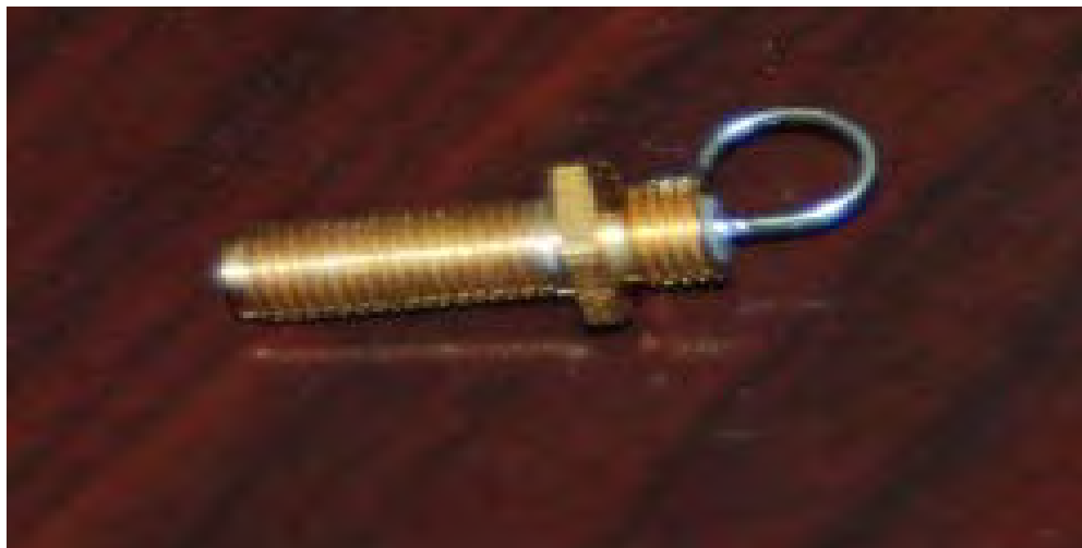
Fig. 4 Standard SMA connected full loop receiver
