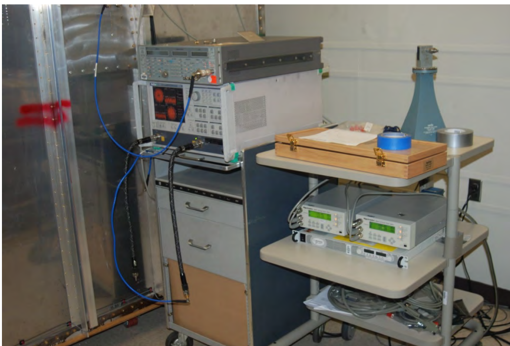
Fig. 9 RF synthesizer, VNA, power meters, and DC power supply
